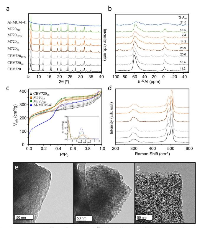
Fig. 1 Structural characterization. (a) X-ray diffraction patterns, (b)  $^{27}$ Al MAS-NMR, (c)  $N_2$  isotherms, (d) Raman spectroscopy of the zeolites prepared. TEM images of (e) CBV720, (f) M720<sub>3h</sub> and (g) Al-MCM-41 materials as representative of microporous and mesoporous materials.
