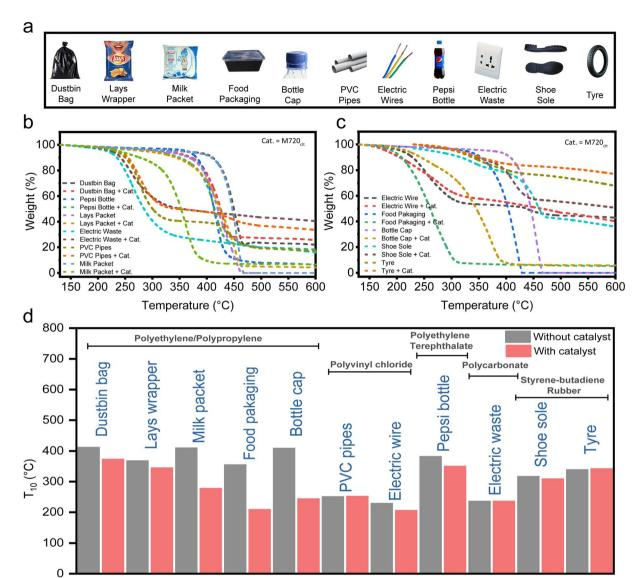
Fig. 5 Plastic waste degradation Study. (a) Different plastic wastes collected from our surroundings. (b and c) Weight loss curves of plastic waste (6 mg each), and using M720<sub>cit</sub> (2 mg). (d) Comparison of  $T_{10}$ 's of different plastic waste used in the study.
