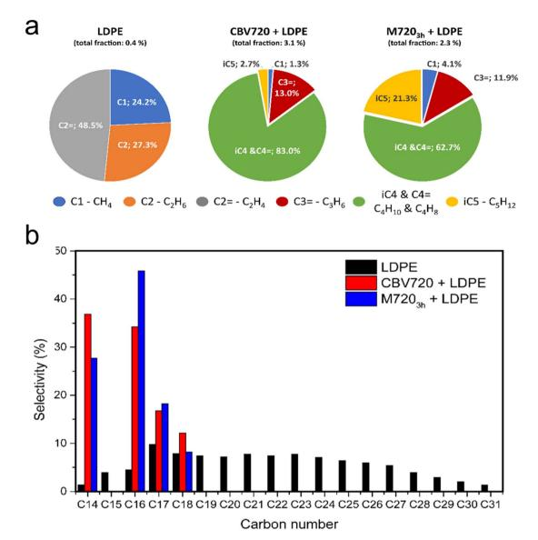
Fig. 4 LDPE cracking profile. (a) Gas fraction and (b) non-volatile compound selectivity analysis.
