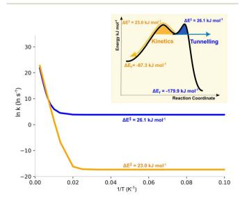
Fig. 3 Arrhenius plot for the two pathways of the decomposition of isomer 178. The inset shows a schematic of the thermodynamic/kinetic/tunnelling control of this species.<sup>36,38</sup>
