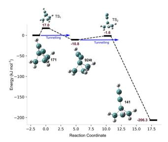
Fig. 4 Potential energy surface for the stepwise, "domino tunnelling" $^{34.50}$  degradation pathway from isomer 171, and their relative energies in kJ  $\mathrm{mol}^{-1}$ .
