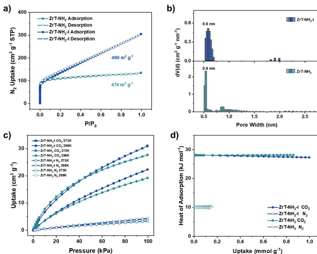
Fig. 4 (a) Nitrogen adsorption (solid symbols) and desorption (hollow symbols) isotherms at 77 K. (b) Pore size distributions calculated from the QSDFT model. (c) CO<sub>2</sub> and N<sub>2</sub> adsorption isotherms at 273 K and 298 K. (d) Isothermic heats of adsorption (Q<sub>st</sub>) calculated from the temperature-dependent CO<sub>2</sub> and N<sub>2</sub> isotherms for the materials of ZrT-NH<sub>2</sub> and ZrT-NH<sub>2</sub>-I.
