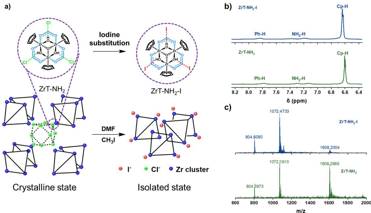
Fig. 1 (a) The synthetic route to ZrT-NH<sub>2</sub>-I. (b) <sup>1</sup>H NMR spectra and (c) ESI-MS spectra of ZrT-NH<sub>2</sub> (green) and ZrT-NH<sub>2</sub>-I (blue).
