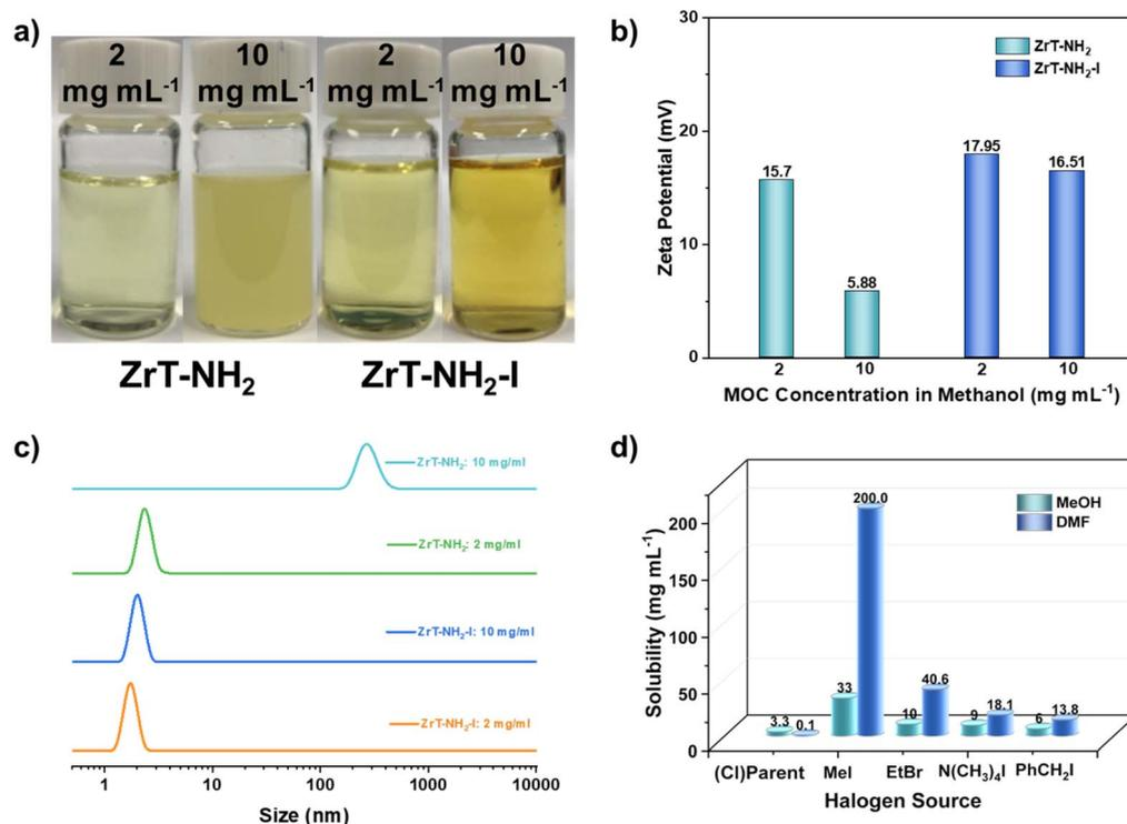
Fig. 3 (a) ZrT-NH<sub>2</sub> and ZrT-NH<sub>2</sub>-I solutions or suspensions with different concentrations. (b and c) Zeta potentials (b) and DLS (c) of ZrT-NH<sub>2</sub> and ZrT-NH<sub>2</sub>-I with different concentrations. (d) The solubility of ZrT-NH<sub>2</sub> (parent material) and its derived materials after reaction with different halogen sources in CH<sub>3</sub>OH (MeOH) and DMF.
