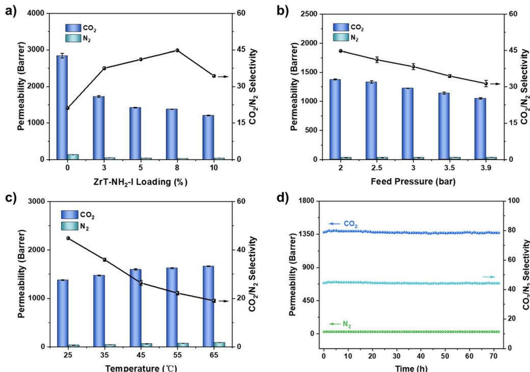
Fig. 7 The effects of (a) ZrT-NH<sub>2</sub>-I loading, (b) feed pressure, (c) test temperature and (d) test time on CO<sub>2</sub> and N<sub>2</sub> permeability and CO<sub>2</sub>/N<sub>2</sub> selectivity.
