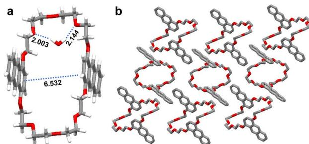
**Fig. 3** (a) Single crystal structure of **An34C10**. Carbon atoms are grey, oxygen atoms are red, and hydrogen atoms are white. Crucial distances are marked with dashed lines. One water molecule was encapsulated in the cavity that might come from a trace amount of water in the solvent. Solvent molecules are omitted for clarity. (b) The packing mode of **An34C10**. Hydrogen atoms and solvents are omitted for clarity.
