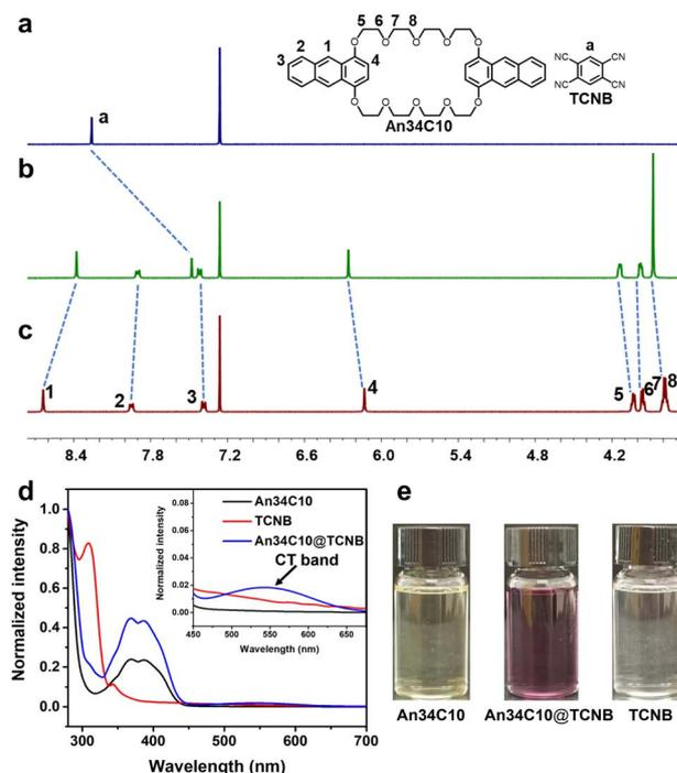
**Fig. 4** <sup>1</sup>H NMR spectra (400 MHz, chloroform-*d*, 298 K): (a) TCNB; (b) 5.00 mM TCNB and 5.00 mM **An34C10**; (c) **An34C10**. (d) Normalized UV-vis absorption spectra (CHCl<sub>3</sub>): **An34C10** (1.00 mM); TCNB (1.00 mM); **An34C10** and TCNB (1.00 mM, each). (e) Photographs: **An34C10** (1.00 mM); TCNB (1.00 mM); **An34C10** and TCNB (1.00 mM, each).
