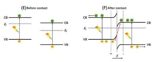
Fig. 11 Charge-transfer route in (A) type I, (B) type II, (C) traditional Z-scheme, and (D) all-solid-state Z-scheme heterojunctions. Adapted from ref. 170 with permission from John Wiley and Sons, copyright 2017. Schematic diagram of energy band changes of semiconductors forming S-type heterojunctions before (E) and after (F) contact. Adapted from ref. 171 with permission from Elsevier, copyright 2020.
