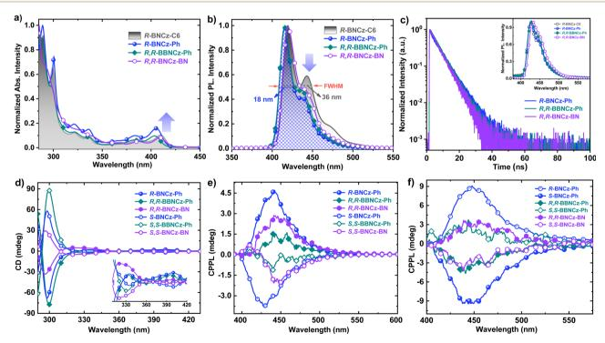
Fig. 2 The (a) UV-Vis absorption and (b) fluorescence spectra of R-BNCz-C6, R-BNCz-Ph, R, R-BBNCz-Ph and R, R-BNCz-BN in dilute toluene (1  $\times$  10<sup>-5</sup> M), (c) transient PL. spectra of these chiral emitters doped in mCBP: DBFPO (1:1) matrix (inset: corresponding steady-state fluorescence spectra) the (d) CD, (e) CPPL spectra of these enantiomers in dilute toluene (1.0  $\times$  10<sup>-5</sup> M) or (f) CPPL spectra in doped thin films.
