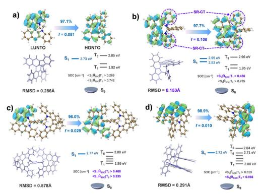
Fig. 3 The NTO analysis, structural difference between the optimized S<sub>1</sub> (light purple) and S<sub>0</sub> (gray), calculated key excited energy levels and relevant SOC values for (a) *R*-BNCz-C6, (b) *R*-BNCz-Ph, (c) *R*,*R*-BBNCz-Ph and (d) *R*,*R*-BNCz-BN.
