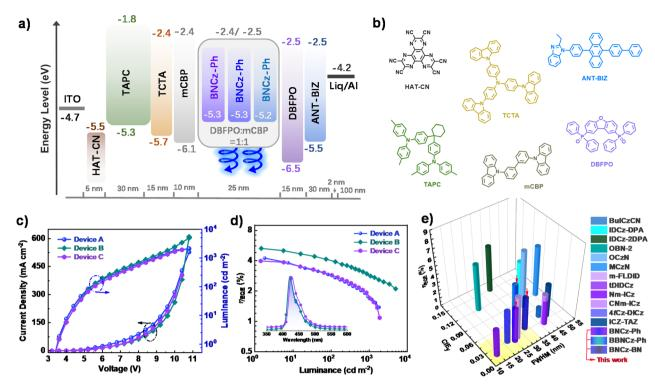
Fig. 6 (a) Schematic illustration of the device architectures and associated energy levels of the constituent materials, (b) the chemical structure of these used materials, (c) the J-V-L curves and (d) the  $\eta_{EQE}$  versus luminance (inset: EL spectra at 6 V) of these devices. (e) Multi-dimensional parallel comparison (involving CIE<sub>y</sub>, FWHM, and  $\eta_{EQE,max}$ ) of the EL performances for MR type blue fluorescence emitters based OLEDs (with  $EL_{Deak} > 400$  nm).
