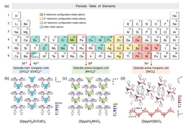
Fig. 1 (a) Periodic table of elements. (b and c) The packing diagrams of the crystal structures of  $(DppyH)_2MCl_4$  ( $M = Zn^{2+}$ ,  $Cd^{2+}$ , and  $Mn^{2+}$ ) along the crystallographic c-axis. (d) The packing diagram of the crystal structure of  $(DppyH)SbCl_4$  along the crystallographic b-axis, and 1D inorganic infinite chain composed of corner-sharing  $[SbCl_5]^{2-}$  pyramids (the blue dashed lines represent hydrogen bonds and partial hydrogen atoms are omitted).
