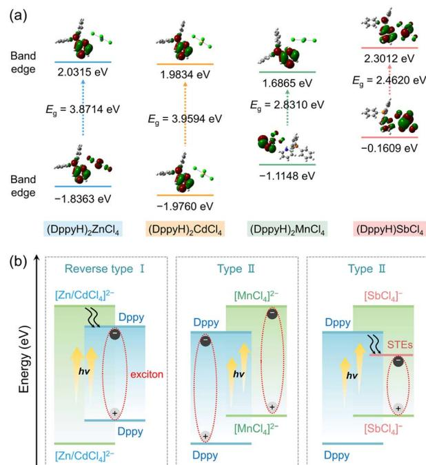
Fig. 4 (a and b) Orbital energy levels and corresponding electronic charge densities for the VBM and CBM as well as band alignments of (DppyH)<sub>n</sub>MCl<sub>4</sub> (M = Zn<sup>2+</sup>, Cd<sup>2+</sup>, Mn<sup>2+</sup>, and Sb<sup>3+</sup>).
