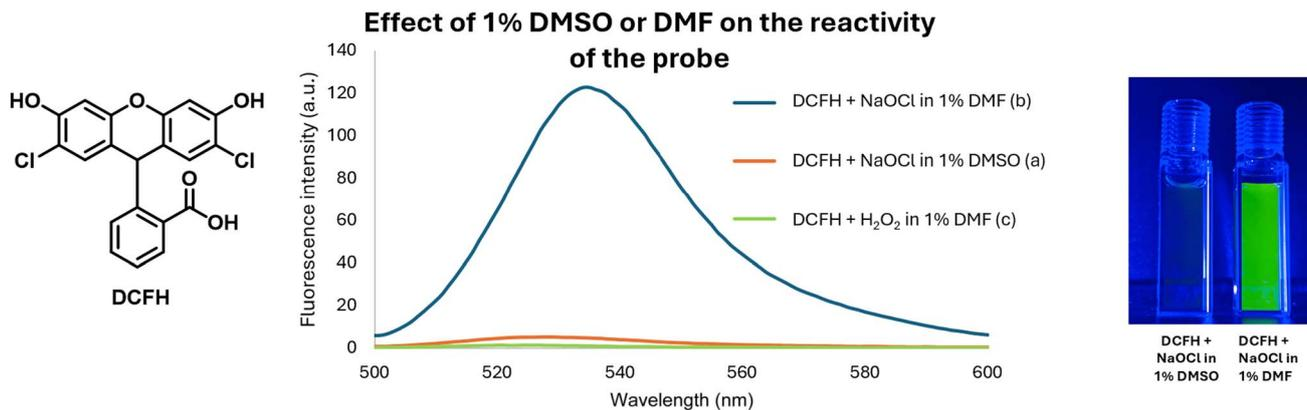
Fig. 4 Effect of 1% DMSO or DMF on the ability for H<sub>2</sub>O<sub>2</sub> and hypochlorite to turn on DCFH fluorescence. (a) Reaction of DCFH (10 μM) with NaOCl (100 μM) in PBS with 1% DMSO at pH 7.4 & 37 °C. (b) Reaction of DCFH (10 μM) with NaOCl (100 μM) in PBS with 1% DMF at pH 7.4 & 37 °C. (c) Reaction of DCFH (10 μM) with H<sub>2</sub>O<sub>2</sub> (100 μM) in PBS with 1% DMF at pH 7.4 & 37 °C.
