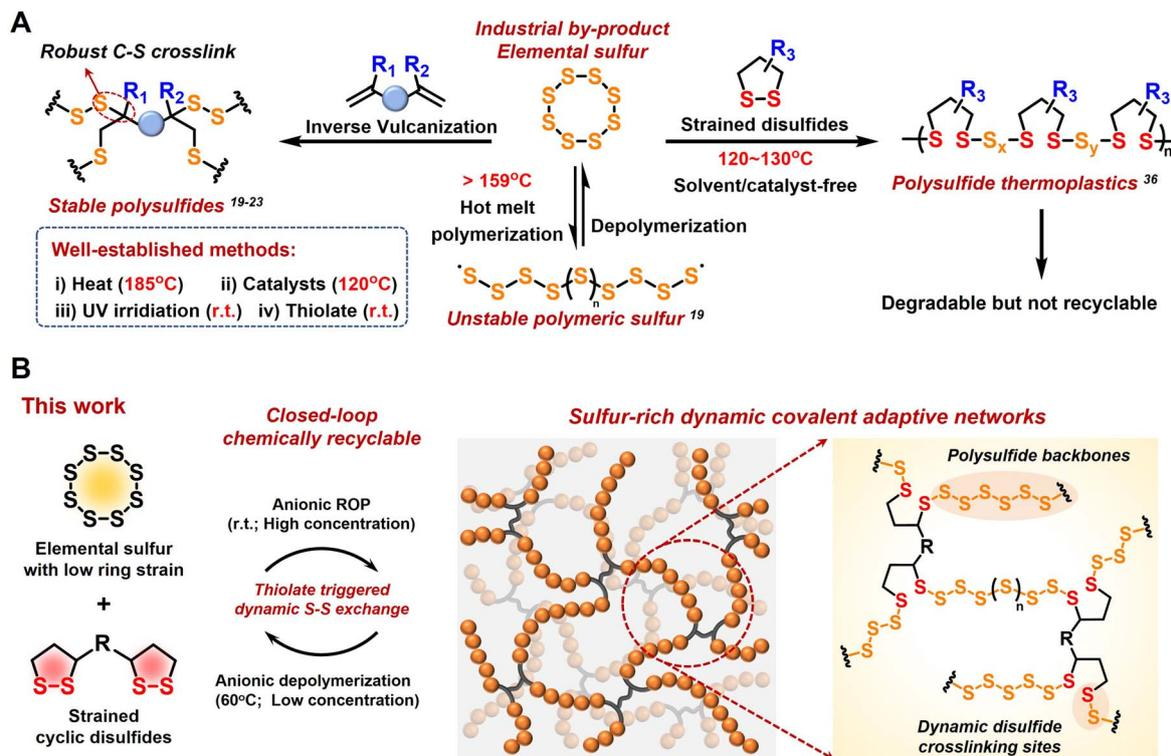
Fig. 1 (A) Considerable advances in the “inverse vulcanization” strategies using S<sub>8</sub> and dienes for innovative polymeric materials. (B) Schematic representation of the anionic copolymerization route of S<sub>8</sub> and cyclic disulfides, yielding sulfur-rich dynamic CANs. The polysulfide backbones and dynamic disulfide crosslinking sites endow the resulting copolymer with reprocessability and chemical recyclability.
