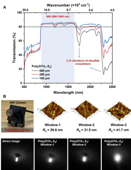
Fig. 4 IR optical application of polysulfide CANs. (A) NIR transmittance spectra of poly(DTA<sub>1</sub>-S<sub>4</sub>) films with different thicknesses. (B) Optical images taken using a NIR camera with and without the poly(DTA<sub>1</sub>-S<sub>4</sub>) window.
