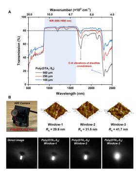
Fig. 4 IR optical application of polysulfide CANs. (A) NIR transmittance spectra of poly(DTA<sub>1</sub>-S<sub>4</sub>) films with different thicknesses. (B) Optical images taken using a NIR camera with and without the poly(DTA<sub>1</sub>-S<sub>4</sub>) window
