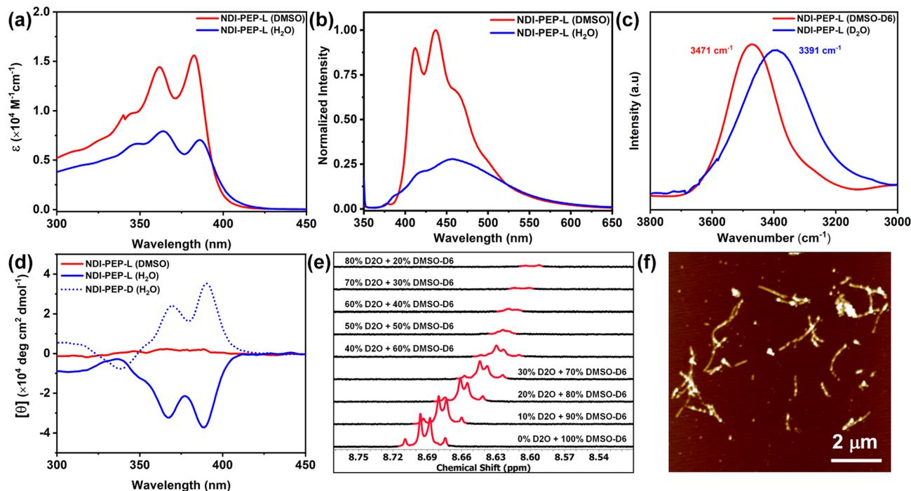
Fig. 1 Solvent-dependent (a) UV-vis spectra; (b) PL spectra; (c) FTIR spectra in the N–H stretching region of NDI-PEP-L; (d) CD spectra of NDI-PEP-L and NDI-PEP-D; (e)  $^1\text{H-NMR}$  spectra of NDI-PEP-L (in the region of aromatic protons) at different % of  $\text{D}_2\text{O}$ ; (f) AFM image of NDI-PEP-L in  $\text{H}_2\text{O}$ . [C = 0.01 mM for UV-vis, PL, CD, and AFM and C = 1 mM for FTIR and NMR studies].
