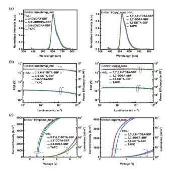
Fig. 3 OLED device performances. (a) Electroluminescence spectra at a luminance of  $1000 \text{ cd m}^{-2}$ , (b) luminance and current density *versus* voltage curves, and (c) EQE and power efficiency *versus* luminance curves of red (left) and green (right) PhOLED devices.
