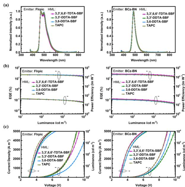
Fig. 4 OLED device performances. (a) Electroluminescence spectra at a luminance of 1000 cd m<sup>-2</sup>, (b) luminance and current density versus voltage curves, and (c) EQE and power efficiency versus luminance curves of blue PhOLED (left) devices and narrowband-emitting BN-MR OLED (right) devices.
