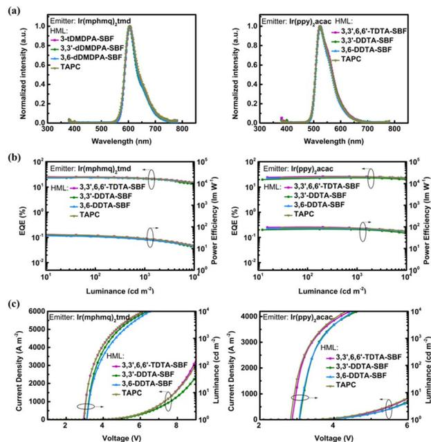
Fig. 3 OLED device performances. (a) Electroluminescence spectra at a luminance of 1000 cd m<sup>-2</sup>, (b) luminance and current density versus voltage curves, and (c) EQE and power efficiency versus luminance curves of red (left) and green (right) PhOLED devices.
