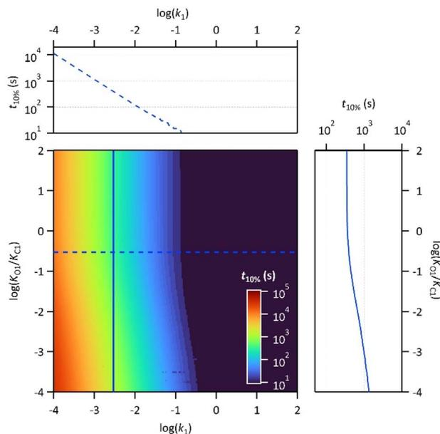
Fig. 5 2D plot of the calculated parameter  $t_{10\%}$  (time required to recover 10% of the OF) as a function of the thermal back reaction kinetic constant  $k_1$  and the ratio of the protonation equilibrium constants  $K_{\text{O}_1}/K_{\text{C}_1}$ . Horizontal and vertical cross-sections are plotted in blue: horizontal cross-section = dotted line for  $K_{\text{O}_1}/K_{\text{C}_1} = 0.3$ ; vertical cross-section = full line for  $k_1 = 3 \times 10^{-3} \text{ s}^{-1}$ .
