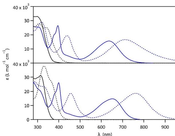
Fig. 2 UV-vis spectra of **1** (top) and **2** (bottom) in the open forms (black curves) and closed forms (blue curves) in acetonitrile, in neutral (full lines) and acidic environment (in the presence of 10 eq. PTSA) (dotted lines).
