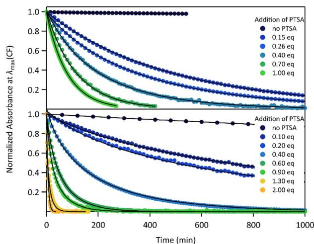
**Fig. 4** Kinetics of the thermal back reaction at 20 °C for **1** (top) and **2** (bottom) in the presence of different PTSA equivalents (full circles), and corresponding curve fits obtained from the kinetic analyses, based on the mechanism shown in Scheme 1 (black lines).
