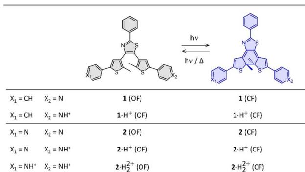
Fig. 1 Photochromic reaction of the compounds studied between the open form (OF) and closed form (CF), in their neutral (**1** and **2**) and protonated (**1**·H<sup>+</sup> and **2**·H<sub>2</sub><sup>2+</sup>) states.
