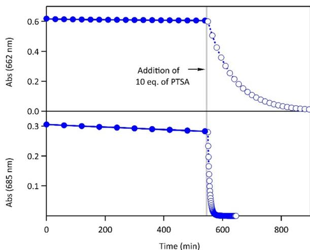
**Fig. 3** Evolution of the absorbance at 662 nm (resp. 685 nm) corresponding to the decay of the CF of **1** (top) and **2** (bottom) at 20 °C in acetonitrile (full circles, neutral environment) and upon addition of 10 eq. of PTSA (open circles, acidic environment), CF was produced beforehand by irradiating the OF at 313 nm. After reaching PSS, irradiation was stopped at time zero.
