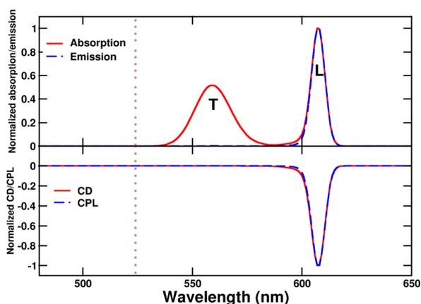
Fig. 7 Spectra calculated for a single C8O3 tube. Upper panel: normalized absorption and emission spectra,  $L$  and  $T$  stand for "transverse" and "longitudinal" polarization, respectively. Lower panel: calculated CD and CPL spectra. The dotted gray line marks the position of the monomer absorption.
