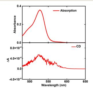
Fig. 3 Absorption (upper panel) and CD spectrum (lower panel) of C8O3 aggregates in thin film, after they have been heated progressively to 388 K until the aggregates are disassembled.
