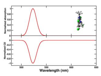
Fig. 5 Normalized absorption (upper panel) and circular dichroism (CD, lower panel) spectra of the twisted chiral C8O3 chromophoric core. A single transition is considered for the monomeric unit (see text), with a Gaussian bandshape and a width  $\sigma=0.045$  eV (*cf.* eqn (S7)).†
