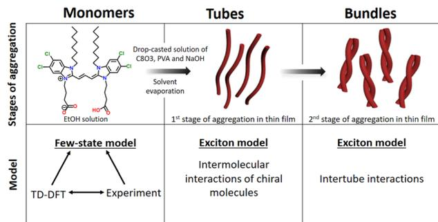
Fig. 1 Upper panels: various stages of aggregation and relevant experimental conditions. Lower panels: theoretical models employed to describe each stage of aggregation.
