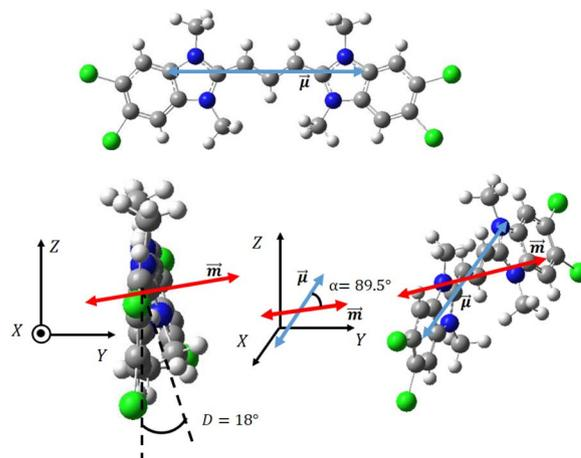
Fig. 4 Upper panel: front view of C8O3 chromophoric core, where the electric transition dipole moment  $\vec{\mu}$  is visible as a double headed blue arrow. Left lower panel: side view of twisted C8O3 chromophoric core, where the magnetic transition dipole moment  $\vec{m}$  is visible as a double-headed red arrow. Right lower panel: the molecular reference system is rotated to showcase the orientation of both the electric and magnetic transition dipole moments.
