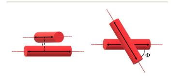
Fig. 8 Side view (left panel) and top view (right panel) of the geometry for the bundle model, where each tube is represented by a red cvlinder.
