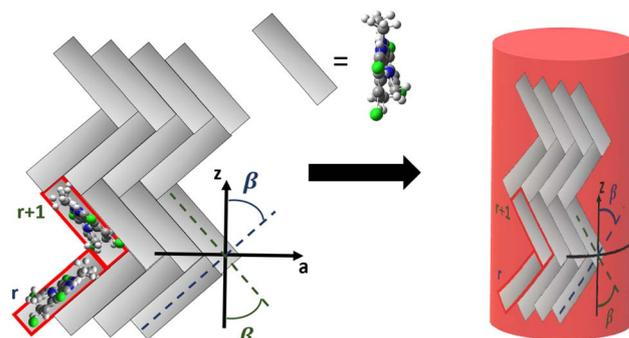
Fig. 6 The herringbone 2D-lattice of C8O3, where cyanines in the  $r$ -th row form a  $\beta$  angle with the positive direction of the  $z$  axis and cyanines in the  $r + 1$ -th row form the same angle with the opposite direction of the  $z$  axis (left), is folded to obtain a tube, with  $z$  becoming the tube axis (right).
