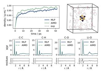
Fig. 2 Validation of MLP. (Top, left) Density of a pure THF system. (Top, right) Simulation box for a sample  $\text{Li}_4\text{X}_4$  system in THF; THF hydrogens omitted for clarity. (Bottom) Radial distribution functions (RDFs) over main atomic pairs.
