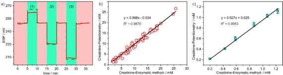
Fig. 5 (a) Expected (dashed line) and experimental (full line) potentiometric response obtained for 1:10 (1), 1:50 (2) and 1:100 (3) dilutions of urine (red) for the sensor. The baseline in between samples (green) corresponds to a 1.0 mM creatinine standard; creatinine values obtained in several urine ((b), N=60) and serum ((c), N=6) samples with the creatinine ion-selective electrode compared with the standard colorimetric standard method – the enzymatic method.
