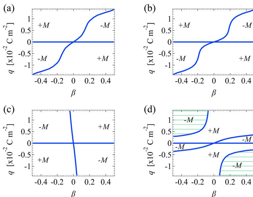
Fig. 8 Diffusioosmotic flow direction of divalent electrolytes versus the channel surface charge density  $q$  and ion diffusivity ratio  $\beta$ . Ion-ion electrostatic correlations are accounted for ( $\delta_c = \kappa l_c$ ). Other figure captions are the same as those in Fig. 7. The shaded regions in (d) are absent in Fig. 7(d), owing to the stronger electrostatic correlations in a divalent electrolyte than a monovalent electrolyte.
