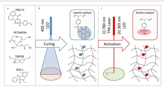
Fig. 1 (a) Components used in the preparation of the thiol—ene formulations. (b) Preparation of dynamic photopolymers by visible light induced radical curing (405 nm) of the thiol—ene monomers and immobilization of the photoacid generator (PAG-Vi). (c) Selective activation of the immobilized PAG-Vi by exposure with (i) two photon absorption laser light at 780 nm or (ii) 365 nm LED light.
