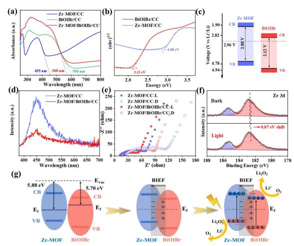
Fig. 4 (a) UV-vis spectrum. (b) Tauc plot. (c) Band structure diagram. (d) PL spectrum. (e) EIS spectra of Zr-MOF/CC and Zr-MOF/BiOIBr/CC with/without illumination. (f) *In situ* XPS spectra under dark and irradiation conditions: Zr 3d. (g) Schematic diagram of directed transfer of photogenerated carriers under the influence of BIEF.
