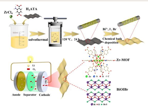
Fig. 1 Schematic diagram of the preparation of Zr-MOF/BiOIBr/CC.
