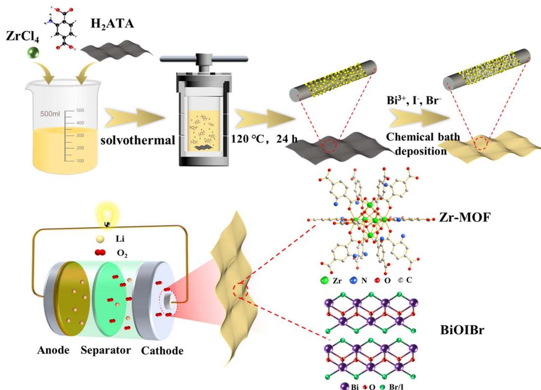
Fig. 1 Schematic diagram of the preparation of Zr-MOF/BiOI/Br/CC.
