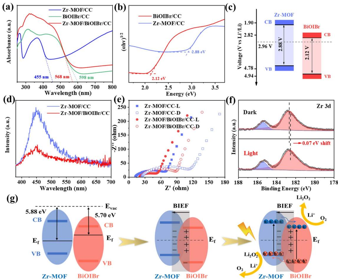
Fig. 4 (a) UV-vis spectrum. (b) Tauc plot. (c) Band structure diagram. (d) PL spectrum. (e) EIS spectra of Zr-MOF/CC and Zr-MOF/BiOI/CC with/without illumination. (f) *In situ* XPS spectra under dark and irradiation conditions: Zr 3d. (g) Schematic diagram of directed transfer of photogenerated carriers under the influence of BIEF.
