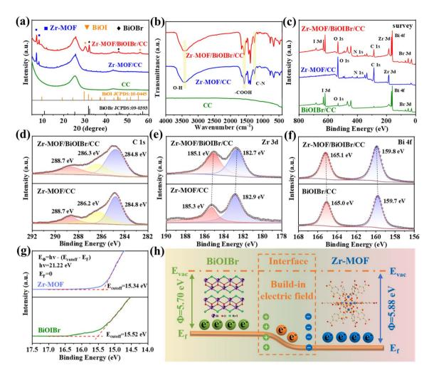
Fig. 3 (a) XRD spectra of CC, Zr-MOF/CC, and Zr-MOF/BiOIBr/CC, (b) FT-IR spectroscopy, XPS of (c) survey, (d) C 1s, (e) Zr 3d, (f) Bi 4f, (g) UPS spectra, and (h) schematic diagram of the formation of BIEF in Zr-MOF and BiOIBr.
