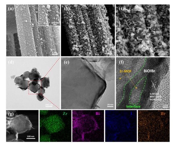
Fig. 2 (a) SEM image of Zr-MOF/CC, (b and c) SEM images of Zr-MOF/BiOIBr/CC, (d-f) TEM images of Zr MOF/BiOIBr, and (g) elemental mappings of Zr, Bi, I, and Br.
