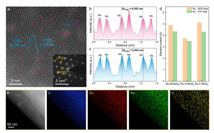
Fig. 3 Atomic structure characterization of  $Ru-O-MoS_2$  catalysts. (a) STEM image of  $Ru-O-MoS_2$ . Inset: the SAED image of  $Ru-O-MoS_2$ . The Ru atoms are marked with red circle dotted line. Atomic height cross sections of (b) Ru-coordinated and (c) pure  $MoS_2$ , respectively.  $d_{(100)}$  denotes the spacing of the (100) crystal planes in the  $MoS_2$  lattice. (d) The content of Ru atoms in each sample based on ICP and XPS data. (e) EDS mapping image of  $Ru-O-MoS_2$ .
