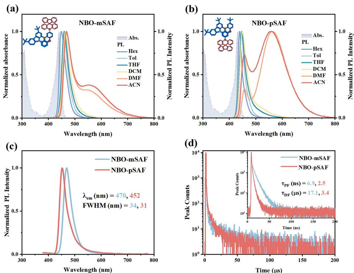
Fig. 3 Normalized UV-vis absorption in dilute toluene ( $10^{-5}$  M) solution and solvatochromic effect on photoluminescence (PL) spectra of (a) NBO-mSAF and (b) NBO-pSAF, and the normalized PL spectra (c) and transient PL decay curves (d) of NBO-mSAF and NBO-pSAF in 6 wt% doped films of 26DCzPPy.
