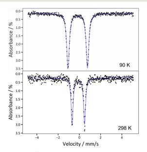
Fig. 3 Zero-field  $^{57}$ Fe Mössbauer spectra of 2 collected at T=90 K (top) and T=298 K (bottom). The blue traces correspond to the overall fits, which are described in the main text.
