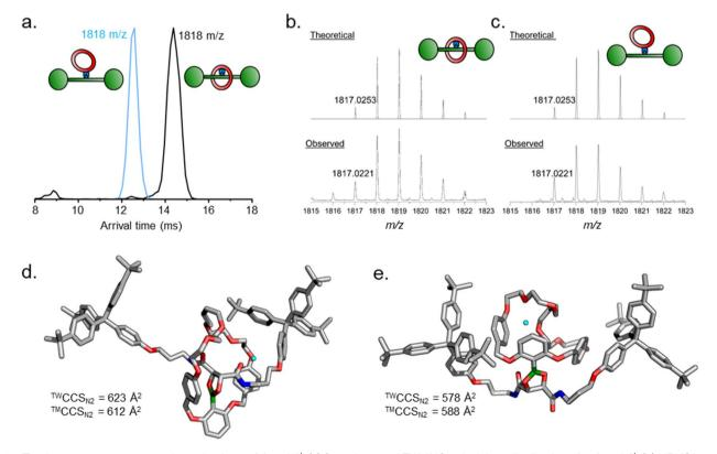
Fig. 3 Tandem mass spectrometry investigations of 4 and 4'. (a) Superimposed TW-IMS arrival time distributions for 4 and 4'. (b) HRMS isotopic distribution for 4. (c) HRMS isotopic distribution for 4'. (d) and (e) HF-3c molecular models for (d)  $[4 \cdot Na]^+$  and (e)  $[4' \cdot Na]^+$  used for calculation of theoretical collisional cross sections (TMCCS<sub>N2</sub>) and comparison with experimental collisional cross section values (TWCCS<sub>N2</sub>). Na<sup>+</sup> ion shown in cyan.
