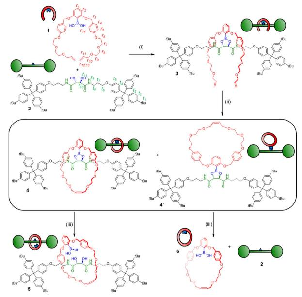
Scheme 1 Synthesis of a [2]rotaxane through boronic acid/diol condensation. Reagents and conditions: (i) 1 (1 equiv.), 2 (1 equiv.), toluene, RT, 24 h; (ii) Hoveyda–Grubbs 2nd generation catalyst,  $CH_2Cl_2$ , RT, 24 h, 16% yield over two steps for 4, 33% yield over two steps for 4'; (iii)  $H_2O$ , CDCl<sub>3</sub>, RT, 1–7 days.
