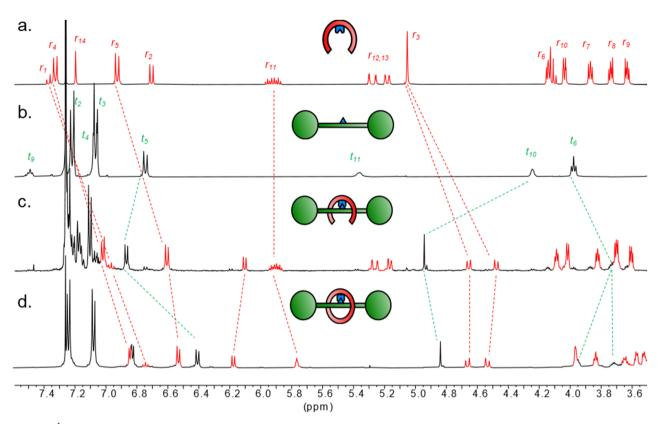
Fig. 1 Partial <sup>1</sup>H NMR spectra (500 MHz, CDCl<sub>3</sub>, 298 K) of (a) boronic acid pincer ligand 1; (b) diol thread 2; (c) boronic ester condensation product 3 (89% conversion); (d) pre-rotaxane 4.
