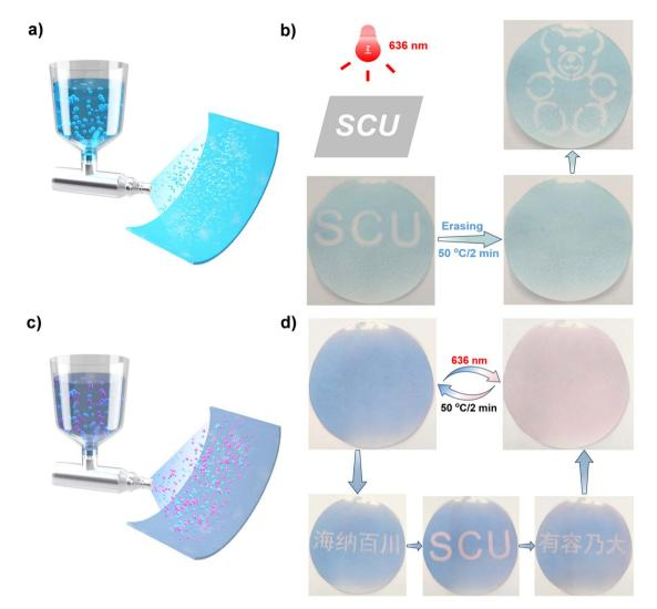
Fig. 4 Schematic illustration of the fabrication of monochromatic rewritable papers using DASA-1 capsules (a) and color-rich rewritable papers using DASA-1 and DASA-2 capsules (c). (b) Photopatterning on the monochromatic paper in a positive manner, with photos captured after photopatterning and erasing. (d) Selective photopatterning on the color-rich paper in a positive manner, with photos captured after photopatterning and erasing
