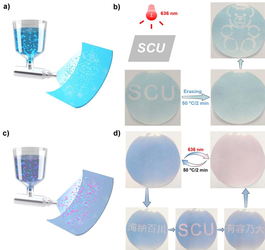
**Fig. 4** Schematic illustration of the fabrication of monochromatic rewritable papers using DASA-1 capsules (a) and color-rich rewritable papers using DASA-1 and DASA-2 capsules (c). (b) Photopatterning on the monochromatic paper in a positive manner, with photos captured after photopatterning and erasing. (d) Selective photopatterning on the color-rich paper in a positive manner, with photos captured after photopatterning and erasing.
