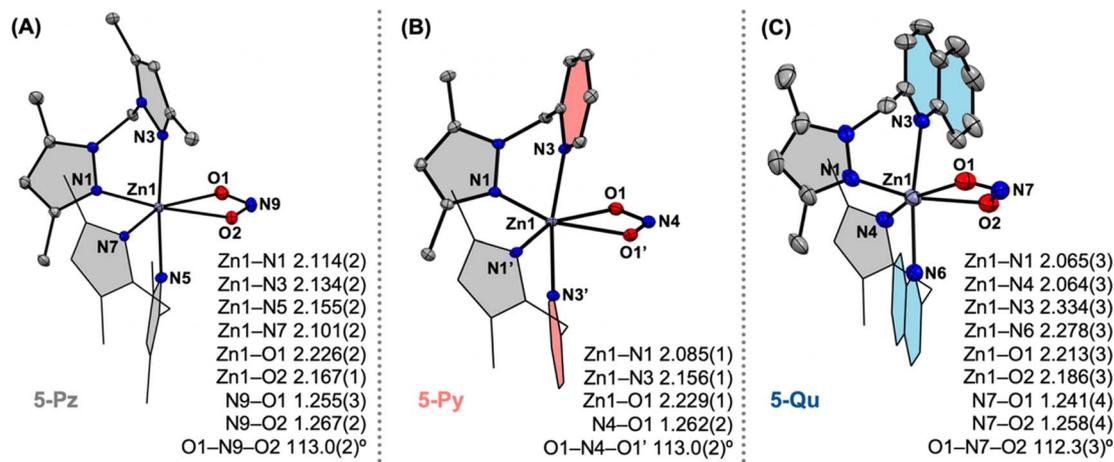
Fig. 6 X-ray crystal structures of the mono-cationic parts of complexes 5-Pz (A), 5-Py (B), and 5-Qu (C). The bond distances tabulated in Å.
