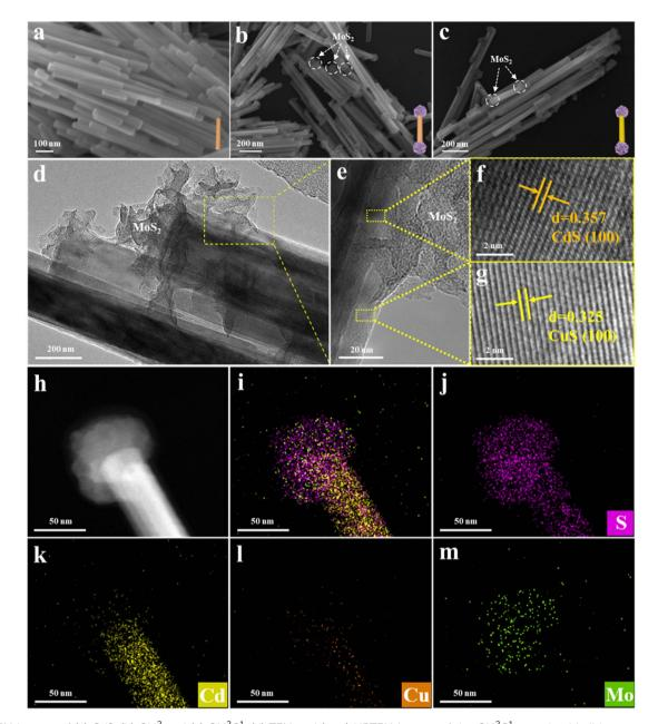
Fig. 1 SEM images of (a) CdS, (b)  $CM^2$  and (c)  $CM^2C^1$ . (d) TEM and (e-g) HRTEM images of the  $CM^2C^1$  nanodumbbell heterostructure, and elemental mapping results of (h-m)  $CM^2C^1$ .
