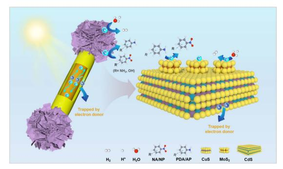
Scheme 2 Schematic illustration of the photocatalytic mechanism of the CdS/MoS<sub>2</sub>/CuS heterostructure.
