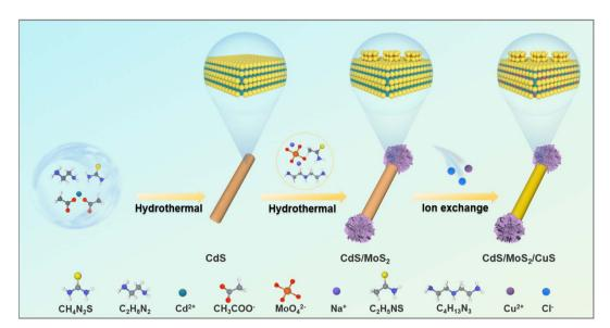
Scheme 1 Schematic illustration depicting the construction of the CdS/MoS<sub>2</sub>/CuS nanodumbbell heterostructure.
