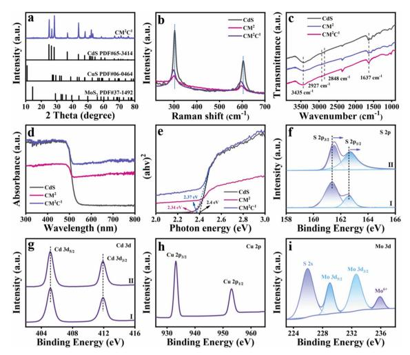
Fig. 2 (a) XRD patterns of the  $CM^2C^1$  nanodumbbell heterostructure; (b) Raman, (c) FTIR, (d) DRS and (e) band-gap determination results of CdS, CM<sup>2</sup> and CM<sup>2</sup>C<sup>1</sup>; high-resolution (f) S 2p and (g) Cd 3d of (I) CdS and (II) CM<sup>2</sup>C<sup>1</sup>; high-resolution (h) Cu 2p and (i) Mo 3d of CM<sup>2</sup>C<sup>1</sup>.
