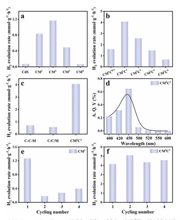
Fig. 3 Photocatalytic hydrogen evolution performances of (a) CdS and CM $^{x}$  (x = 1, 2, 3, 4), and (b) CM $^{2}$ C $^{x}$  (x = 0.5, 1, 2, 3, 4). (c) Photocatalytic hydrogen evolution performances of C-C-M, C/C/M and CM $^{2}$ C $^{1}$ ; (d) A.Q.Y result of CM $^{2}$ C $^{1}$  under monochromatic light irradiation; photostability measurements of (e) CM $^{2}$  and (f) CM $^{2}$ C $^{1}$ .
