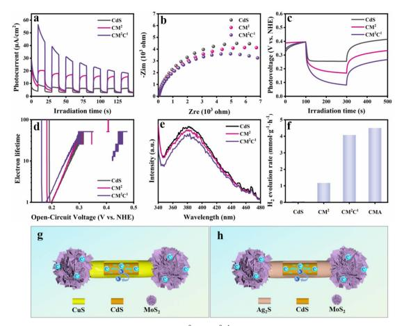
Fig. 5 (a) I-t, (b) EIS, (c) OCVD and (d) electron lifetime of CdS, CM<sup>2</sup> and CM<sup>2</sup>C<sup>1</sup> under visible light ( $\lambda$  > 420 nm) irradiation, (e) PL results of CdS, CM<sup>2</sup> and CM<sup>2</sup>C<sup>1</sup>, (f) photocatalytic hydrogen evolution performances of CdS, CM<sup>2</sup> and CMA, and schematic diagram of photoelectron transfer over the (g) CdS/MoS<sub>2</sub>/CuS and (h) CdS/MoS<sub>2</sub>/Ag<sub>2</sub>S heterostructure.
