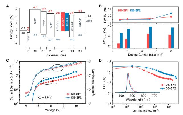
Fig. 5 (A) Device configurations and energy-level diagrams of the non-sensitized devices. (B) Maximum external quantum efficiency (EQE<sub>max</sub>) and full width at half maximum (FWHM) versus dopant concentration relationships of the devices. (C) Current density-voltage-luminance curves and (D) EQE-luminance curves of DB-SF1 and DB-SF2-based OLEDs with 5 wt% doping ratio (inset: electroluminescence spectra at 6 V).
