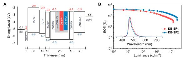
Fig. 6 (A) Device configurations and energy-level diagrams of the hyperfluorescence (HF) devices. (B) EQE-luminance curves with electroluminescence spectra at 6 V as the inset.
