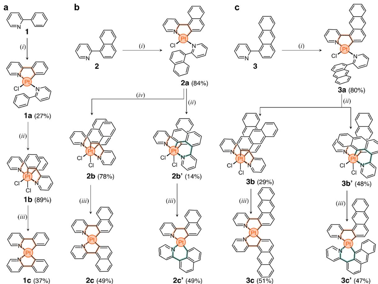
**Scheme 1** Synthesis of cyclometalated Pt complexes using (a) phenyl-, (b) naphthalenyl-, and (c) anthracenylpyridine ligands **1**, **2**, and **3**. Reaction conditions: (i)  $K_2[PtCl_4]$ ,  $H_2O$ , 2-ethoxyethanol, 80 °C,  $N_2$ ; (ii)  $PhICl_2$ , DCM, 25 °C; (iii)  $t-BuOK$ , THF, 60 °C,  $N_2$ ; (iv)  $PhICl_2$ , 1,1,2,2-tetrachloroethane, 130 °C.
