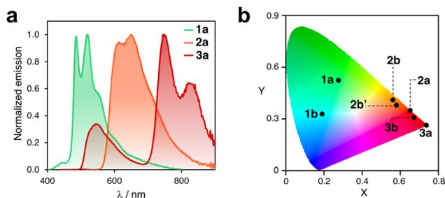
Fig. 5 (a) Emission spectra of complexes **1a**, **2a**, and **3a** in  $\text{DCM}$  at  $25^\circ\text{C}$ . (b) CIE plot of selected  $\text{Pt}^{\text{II}}$  and  $\text{Pt}^{\text{IV}}$  cyclometalated complexes containing ligands **1**, **2** and **3**. Data corresponding to  $\text{DCM}$  solutions recorded at  $25^\circ\text{C}$ .
