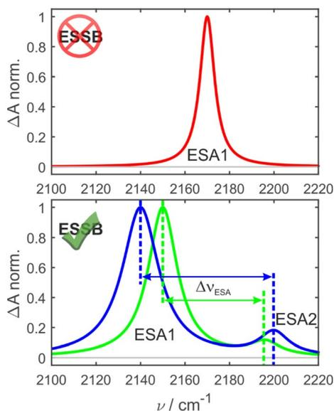
Fig. 2 Schematic principle of the experiment. In the symmetry-preserved excited state (top) there is a single  $C\equiv N$  band (ESA1). Upon symmetry breaking a second band (ESA2) emerges. The splitting between the bands ( $\Delta\nu_{ESA}$ ) increases with asymmetry as schematically illustrated by the green and blue spectra.
