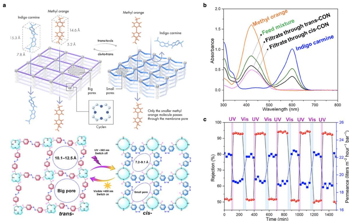
Fig. 8 (a) Schematic illustration of the *trans*–*cis* photoisomerization and chemical structures of the light-responsive membranes. (b) Separation performance of mixed dyes through *trans*- and *cis*-CON membranes. (c) Indigo carmine separation performance in consecutive cycles under UV/vis light. Reproduced with permission from ref. 113. Copyright 2022, American Association for the Advancement of Science.
