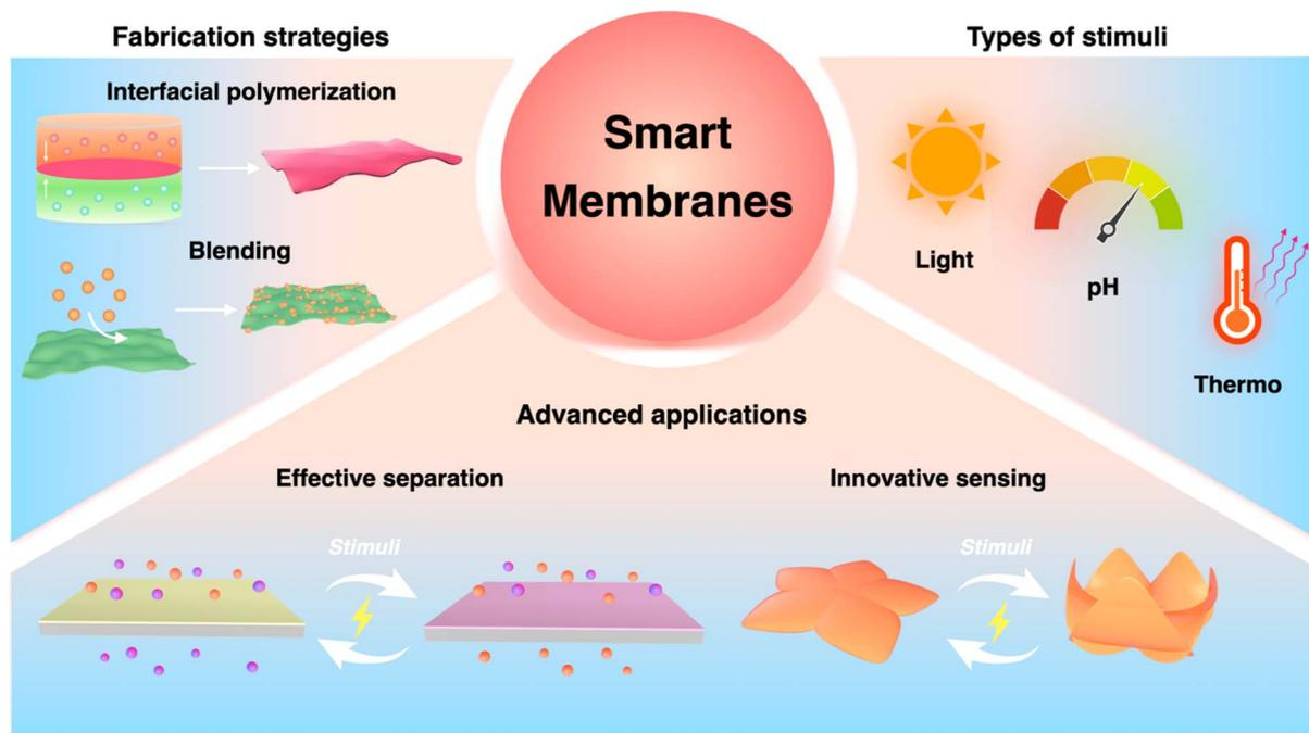
Fig. 1 Schematic illustration of the smart membrane fabrication strategies, types of stimuli, and advanced applications in separations and sensing.
