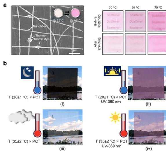
Fig. 7 (a) SEM image of PDMS/Tdye- $\text{Al}_2\text{O}_3$  HNTs and a thermo-dependent color change of the membrane before and after stretching. Reproduced with permission from ref. 105. Copyright 2020, American Chemical Society. (b) Photographic images demonstrate a visual change in transmission and color on exposure to various conditions of temperature and/or UV light. Reproduced with permission from ref. 106. Copyright 2021, American Chemical Society.
