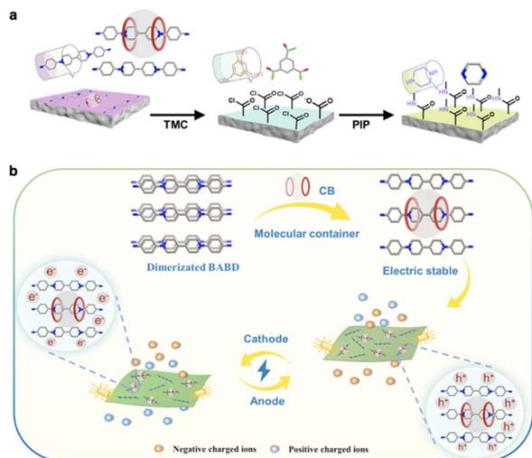
Fig. 3 (a) Schematic preparation of a (CB[7])-viologen membrane *via* interfacial polymerization. (b) Schematic illustration of smart separation achieved by the voltage-gated membrane in the electric field. Reproduced with permission from ref. 56. Copyright 2022, American Chemical Society.
