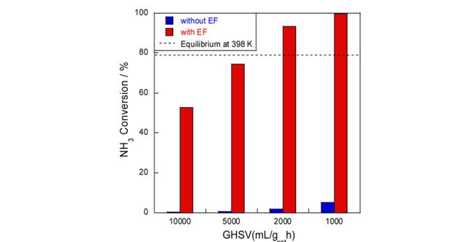
Fig. 2 SV dependence of NH<sub>3</sub> conversion at 398 K over 8.2 mol% Ru/CeO<sub>2</sub>: 300 mg catalyst, 0.1 MPa, and 6.0 mA.
