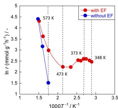
Fig. 3 Arrhenius plots for ammonia decomposition rates over 0.85 mol% Ru/CeO<sub>2</sub>: 5% NH<sub>3</sub>/Ar = 200 SCCM, 200 mg cat, 0.1 MPa, and 0 or 6.0 mA.
