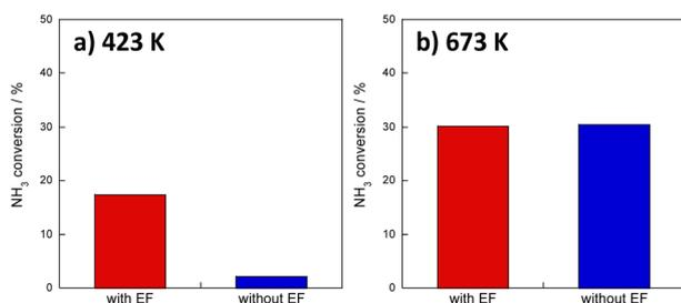
Fig. 1 Temperature dependence of NH<sub>3</sub> decomposition over 8.2 mol% Ru/CeO<sub>2</sub> with and without an electric field: feed, 100% NH<sub>3</sub>, 50 SCCM; catalyst, 100 mg, 0.1 MPa, 0 or 6.0 mA; (a) at 423 K and (b) at 673 K.
