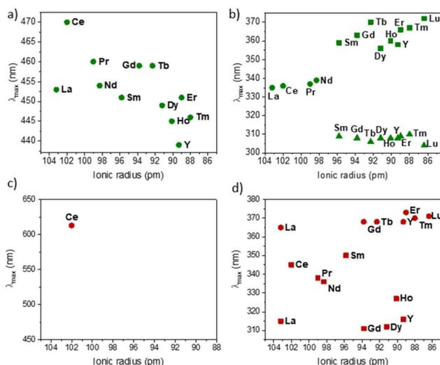
Fig. 8 Evolution of the maximum absorption of 2-Ln (the *cis/trans* ratio is given in Table 3) complexes wavelength around (a) 450 nm and (b) 300–370 nm and of 2-Ln-*cis* (made from the methodology proposed in literature<sup>9,40</sup> around) (c) 400–650 nm and (d) 300–380 nm.
