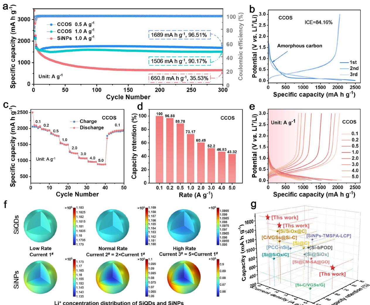
Fig. 4 (a) Cycling performance of CCOS and SiNPs at  $1.0 \text{ A g}^{-1}$ , and CCOS at  $0.5 \text{ A g}^{-1}$ . (b) Initial (dis)charge curves. (c) Rate performance, (d) capacity retention and (e) (dis)charge curves at different rates. (f) COMSOL simulation diagrams of the  $\text{Li}^+$  concentration distribution of SiQDs and SiNPs during the lithiation process at different currents. (g) Ragone plots comparing CCOS with reported silicon-based anodes.<sup>22,39,S1–S8†</sup>
