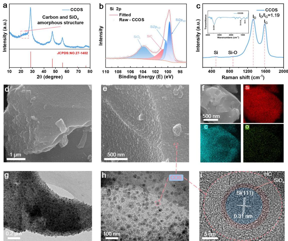
Fig. 2 Structure and composite characterization of CCOS. (a) XRD pattern. (b) The Si 2p high-resolution XPS spectrum. (c) Raman and FTIR (inset) spectra. (d and e) SEM images at different magnifications. (f) SEM-based EDS mapping of Si, C, and O. (g and h) TEM images at different magnifications. (i) HRTEM image.
