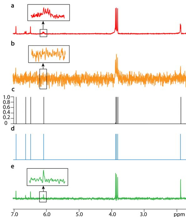
Fig. 3 1D NMR spectra of 1 mM (a, b, and d) and 30 mM  $\alpha$ -asarone (e) dissolved in chloroform- $d$  ( $\text{CDCl}_3$ ) with a scan number of one. (a) The spin echo spectrum with an echo time of 0 s. (b) The PSYCHE spectrum. (c) The confidence result produced by SE2CSNet. (d) The output chemical shift spectra produced by SE2CSNet. (e) The PSYCHE spectrum as a reference. Representative regions are expanded.
