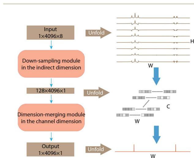
Fig. 1 The architecture of SE2CSNet. The data size is represented by  $C \times W \times H$ , where  $W$  is the size in the direct dimension or the width of the feature matrix,  $H$  is the size in the indirect dimension or the height of the feature matrix, and  $C$  is the number of channels.
