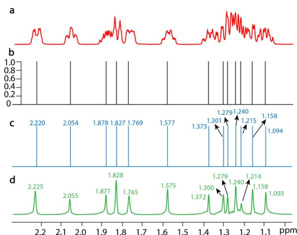
Fig. 2 1D NMR spectra of 50 mM estradiol dissolved in (methyl sulfide)-d6 (DMSO-d6) with a scan number of one. (a) The spin echo spectrum with an echo time of 0 s. (b) The confidence result produced by SE2CSNet. (c) The output chemical shift spectra produced by SE2CSNet. (d) The PSYCHE spectrum as a reference.
