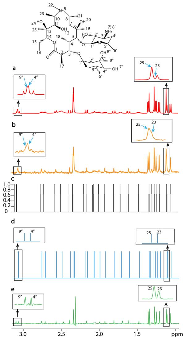
Fig. 5 1D NMR spectra of 20 mM (a, b, and d) and 40 mM azithromycin (e) dissolved in chloroform- $d$  ( $CDCl_3$ ) with a scan number of one. (a) The spin echo spectrum with an echo time of 0 s. (b) The PSYCHE spectrum. (c) The confidence result produced by SE2CSNet. (d) The output chemical shift spectra produced by SE2CSNet. (e) The PSYCHE spectrum as a reference. Representative regions are expanded. Blue arrows indicate representative signals.
