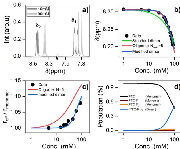
Fig. 5 (a)  ${}^1\text{H}$  NMR chemical shifts showing two distinct environments for the protons ( $\delta_1$  and  $\delta_2$ ) (see ESI†). (b)  ${}^1\text{H}$  NMR chemical shift of PTC as a function of concentration, along with the fit to dimers and oligomers with a maximum cutoff of  $N = 5$ . (c) Effective radius ( $r_{\text{eff}}$ ) extracted from DOSY measurements fit with the same models. (d) Species populations for the modified dimer model.
