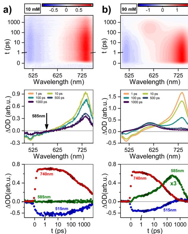
Fig. 3 Transient absorption spectra of PTC in the fs-to-ns window: time-spectral map, gated-spectra at 1, 10, 100, 500, and 1000 ps, and kinetics at 515, 585, and 740 nm for (a) 10 mM, (b) 90 mM solution. Excitation: 415 nm; power: 100 mW.
