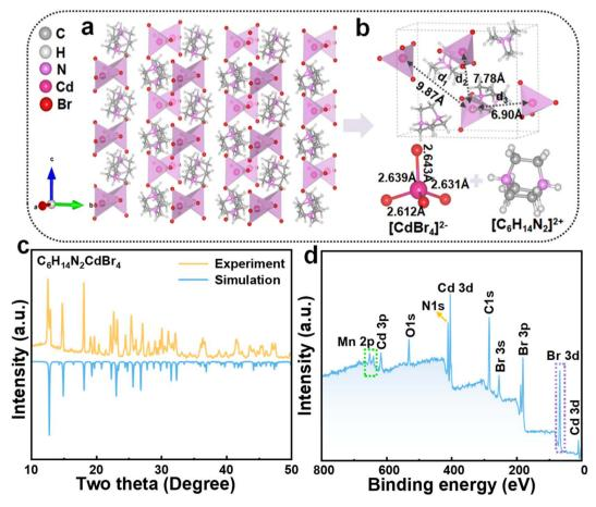
Fig. 1 (a) Structure diagram of the 0D single crystal  $C_6H_{14}N_2CdBr_4$ . (b) The detailed diagram of the different distances between the  $[CdBr_4]^{2-}$  tetrahedra and ball-and-stick diagram of an individual  $[CdBr_4]^{2-}$  unit and organic cation. (c) The experimental and simulated XRD patterns of  $C_6H_{14}N_2CdBr_4$ . (d) XPS full spectrum of  $C_6H_{14}N_2CdBr_4$ :Mn<sup>2+</sup>.
