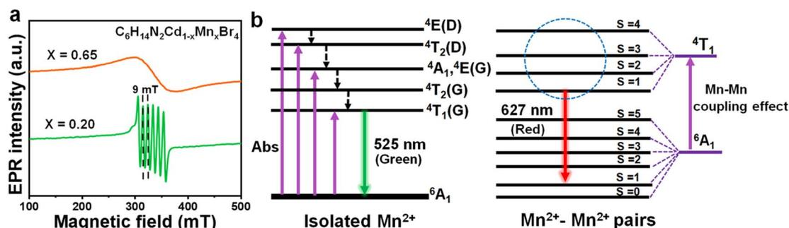
Fig. 3 (a) EPR spectra of  $Mn^{2+}$ -doped  $C_6H_{14}N_2Cd_{1-x}Mn_xBr_4$  with different dopant concentrations. (b) Schematic illustration of the energy levels and optical transitions in the tetrahedrally coordinated isolated  $Mn^{2+}$  ions and the  $Mn^{2+}$ - $Mn^{2+}$  pairs.
