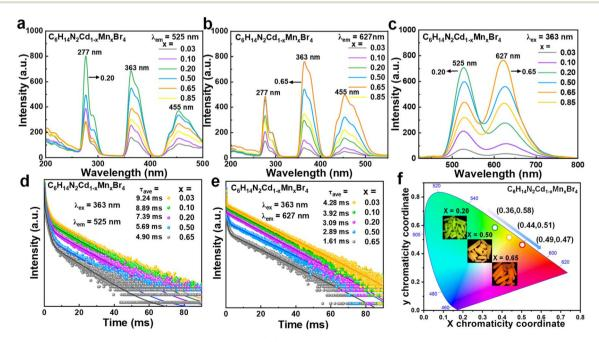
Fig. 2 (a and b) PLE, (c) PL spectra, (d and e) decay curves, and (f) CIE color coordinates of  $C_6H_{14}N_2Cd_{1-x}Mn_xBr_4$  crystals changing with the x value, respectively (the insets are the corresponding photographs of the  $Mn^{2+}$ -doped samples under a 365 nm UV lamp).
