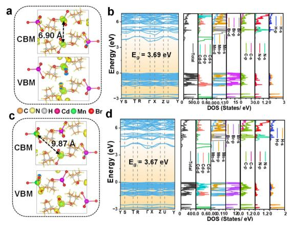
Fig. 4 Charge density distribution of the CBM and VBM, and calculated electronic band structure and partial density of states of  $C_6H_{14}N_2-Cd_{0.50}Mn_{0.50}Br_4$  with different  $Mn^{2+}-Mn^{2+}$  distances at (a and b) 6.90 Å and (c and d) 9.87 Å.
