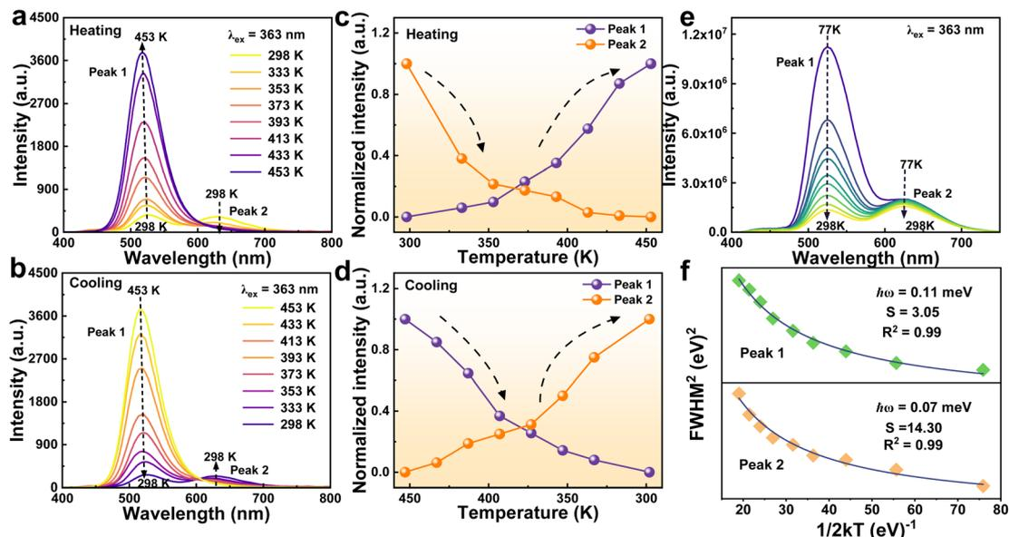
Fig. 6 (a and b) Temperature-dependent emission spectra of  $C_6H_{14}N_2Cd_{0.50}Mn_{0.50}Br_4$  during the heating and cooling processes. (c and d) The corresponding normalized integrated PL intensity of peak 1 and peak 2 at various temperatures during heating and cooling, respectively. (e) PL spectra and the corresponding (f) FWHM of  $C_6H_{14}N_2Cd_{0.50}Mn_{0.50}Br_4$  crystals varied from 77 to 298 K.
