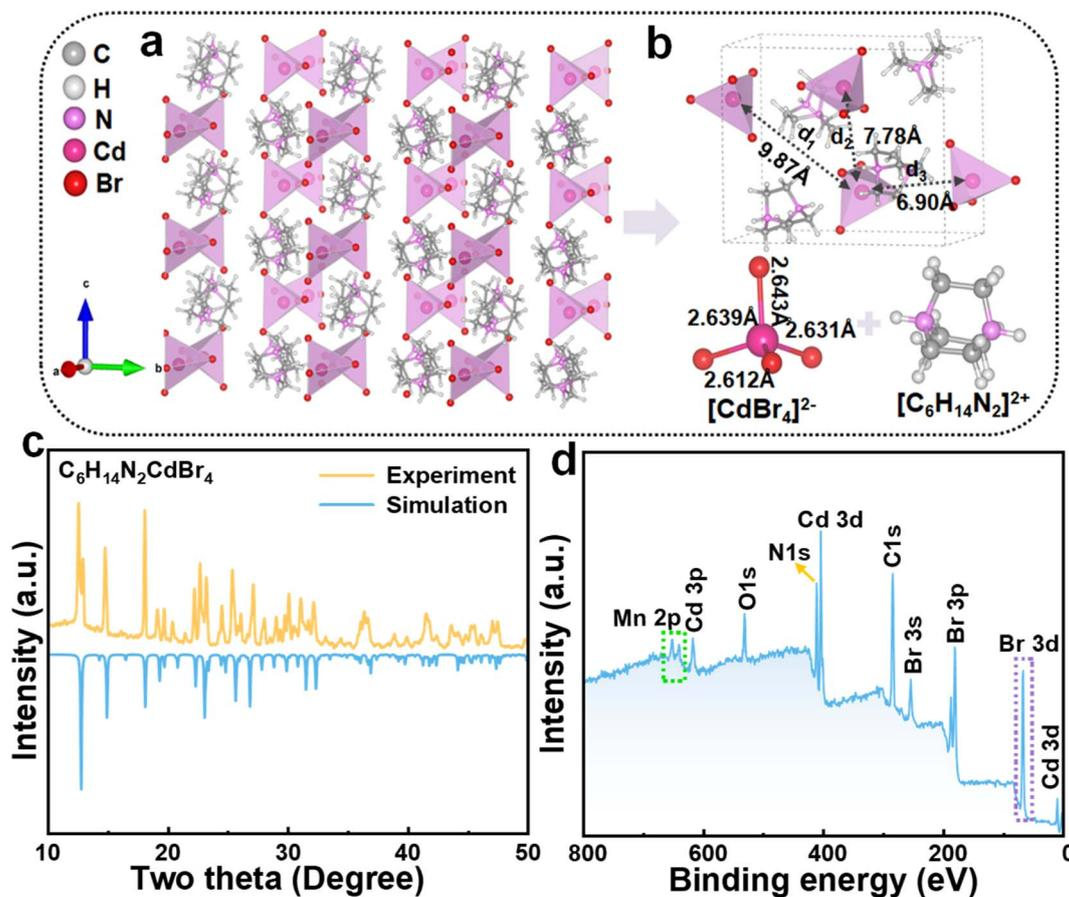
Fig. 1 (a) Structure diagram of the 0D single crystal  $C_6H_{14}N_2CdBr_4$ . (b) The detailed diagram of the different distances between the  $[CdBr_4]^{2-}$  tetrahedra and ball-and-stick diagram of an individual  $[CdBr_4]^{2-}$  unit and organic cation. (c) The experimental and simulated XRD patterns of  $C_6H_{14}N_2CdBr_4$ . (d) XPS full spectrum of  $C_6H_{14}N_2CdBr_4:Mn^{2+}$ .
