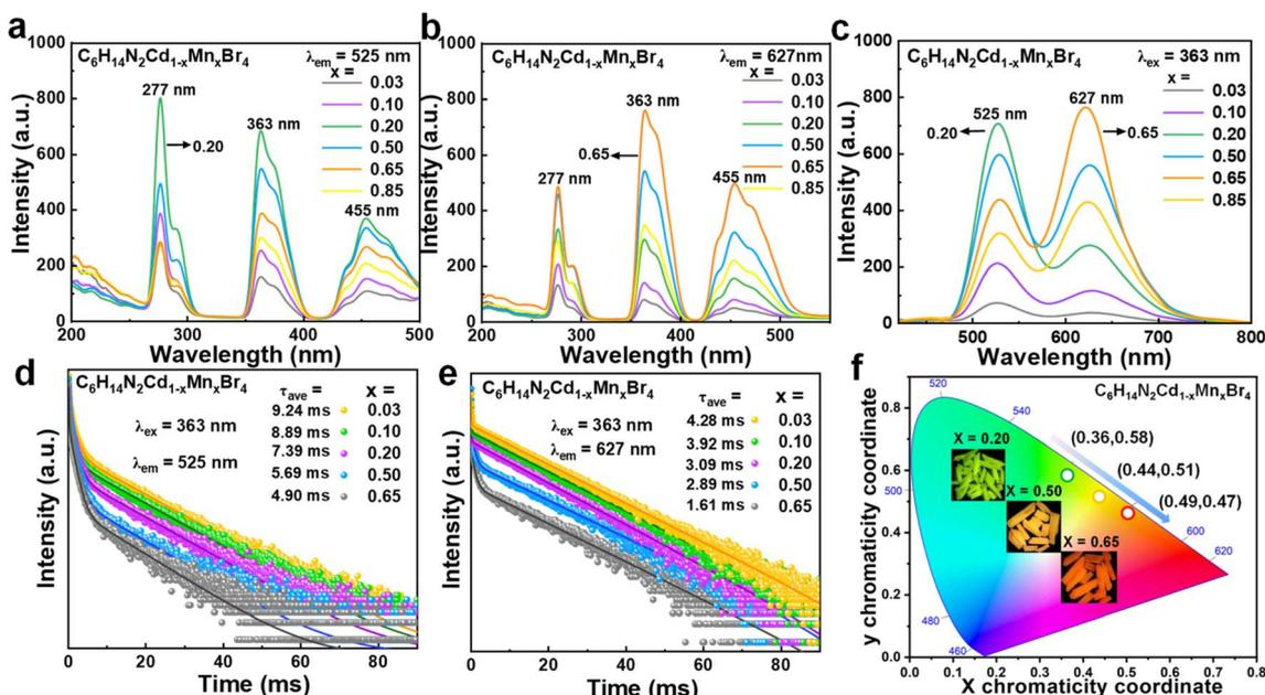
Fig. 2 (a and b) PLE, (c) PL spectra, (d and e) decay curves, and (f) CIE color coordinates of  $\text{C}_6\text{H}_{14}\text{N}_2\text{Cd}_{1-x}\text{Mn}_x\text{Br}_4$  crystals changing with the  $x$  value, respectively (the insets are the corresponding photographs of the  $\text{Mn}^{2+}$ -doped samples under a 365 nm UV lamp).
