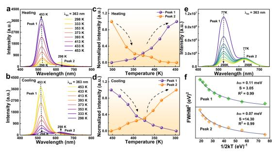
Fig. 6 (a and b) Temperature-dependent emission spectra of  $C_6H_{14}N_2Cd_{0.50}Mn_{0.50}Br_4$  during the heating and cooling processes. (c and d) The corresponding normalized integrated PL intensity of peak 1 and peak 2 at various temperatures during heating and cooling, respectively. (e) PL spectra and the corresponding (f) FWHM of  $C_6H_{14}N_2Cd_{0.50}Mn_{0.50}Br_4$  crystals varied from 77 to 298 K.
