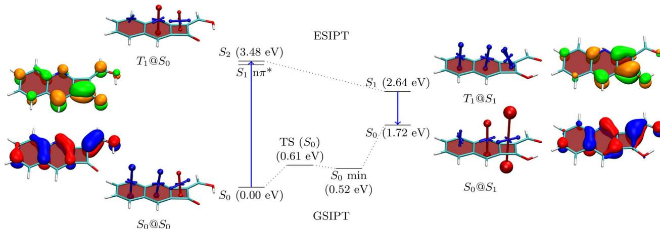
Fig. 3 Analysis of proton transfer induced ESA gain for molecule **3a**. The quinoidal (Q) and (anti)aromatic (A) forms are shown to the left and right, respectively. Energies are given in parentheses. Next to the energies VIST plots as well as the NTOs (blue/red for hole and orange/green for electron) are shown.
