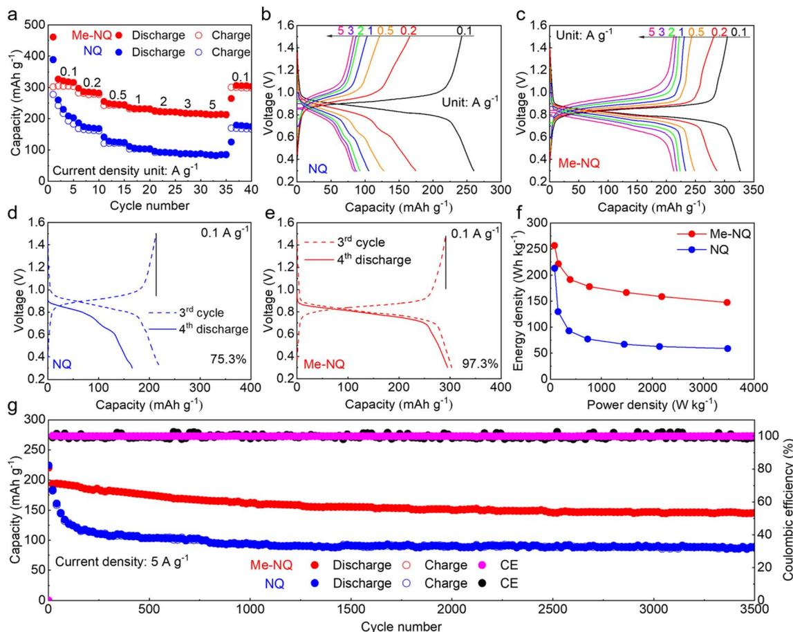
Fig. 2 (a) Rate performance of Me-NQ and NQ. Charge–discharge curves at different current densities of (b) NQ and (c) Me-NQ. Self-discharge tests of (d) NQ and (e) Me-NQ (resting at the charged state for 48 h). (f) Ragone plots (based on active material mass loading) of Me-NQ and NQ. (g) Cycling performance of Me-NQ and NQ at a current density of 5 A g<sup>-1</sup>.
