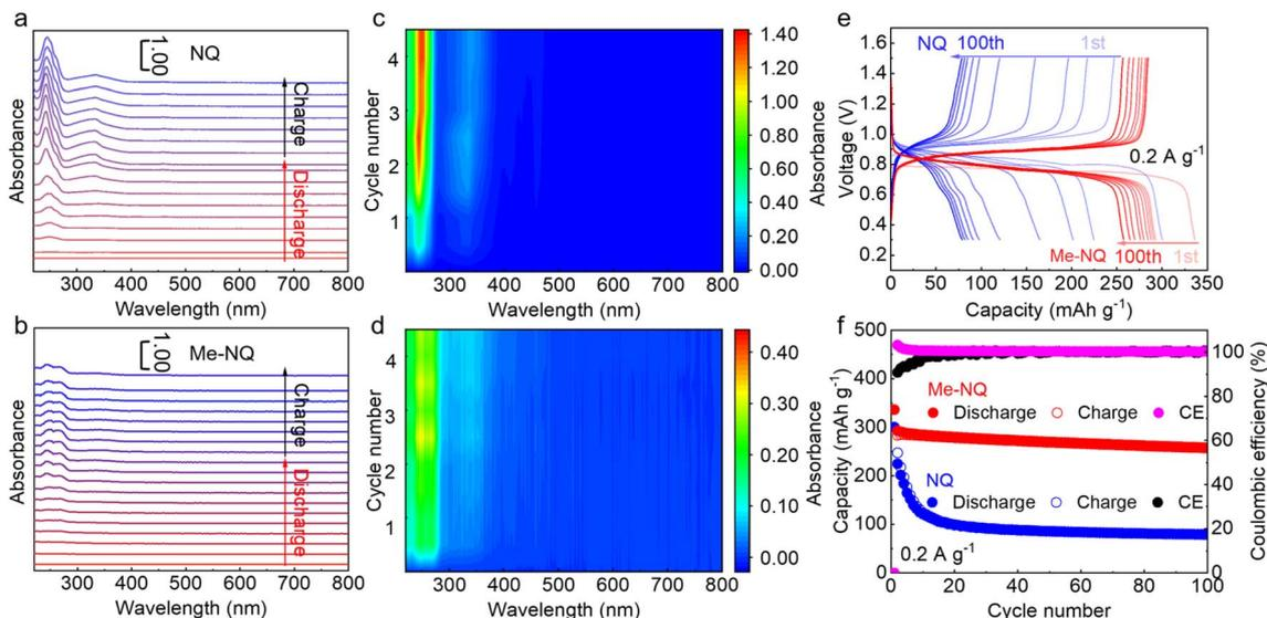
Fig. 3 *In situ* UV-vis spectra of the first cycle of the 2 M ZnSO<sub>4</sub> electrolyte with (a) NQ and (b) Me-NQ cathodes at 0.2 A g<sup>-1</sup>. *In situ* UV-vis spectra of the 2 M ZnSO<sub>4</sub> electrolyte with (c) NQ and (d) Me-NQ cathodes at 0.5 A g<sup>-1</sup>. (e) Charge/discharge curves at different cycles and (f) capacity evolutions of Me-NQ and NQ at 0.2 A g<sup>-1</sup> with active material loading around 4 mg cm<sup>-2</sup>.
