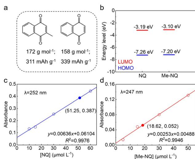
Fig. 1 (a) Molecular structures of Me-NQ (left) and NQ (right). (b) Calculated frontier molecular orbital energy levels of Me-NQ and NQ. UV-vis analysis to calculate the solubilities in 2 M ZnSO<sub>4</sub>: the calibration curves and absorbance of 10 times diluents of saturated (c) NQ and (d) Me-NQ.
