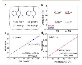
Fig. 1 (a) Molecular structures of Me-NQ (left) and NQ (right). (b) Calculated frontier molecular orbital energy levels of Me-NQ and NQ. UV-vis analysis to calculate the solubilities in 2 M  $\rm ZnSO_4$ : the calibration curves and absorbance of 10 times diluents of saturated (c) NQ and (d) Me-NQ.
