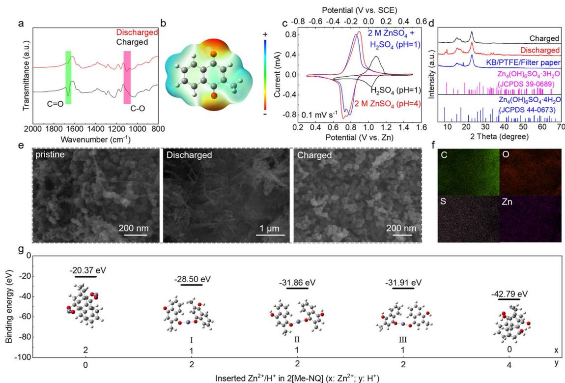
Fig. 5 (a) FT-IR of Me-NQ at different states. (b) ESP map of Me-NQ. (c) CV of Me-NQ in different electrolytes at  $0.1\text{ mV s}^{-1}$ . (d) XRD patterns and (e) SEM images of Me-NQ at different states. (f) EDS mappings of the discharged Me-NQ. (g) Binding energies of two Me-NQ molecules with different numbers of  $\text{Zn}^{2+}$  and  $\text{H}^+$ .
