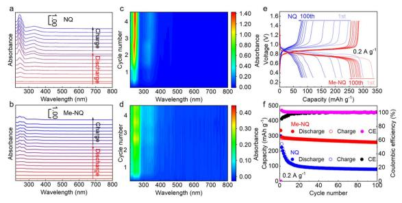
Fig. 3 In situ UV-vis spectra of the first cycle of the 2 M ZnSO<sub>4</sub> electrolyte with (a) NQ and (b) Me-NQ cathodes at 0.2 A  $g^{-1}$ . In situ UV-vis spectra of the 2 M ZnSO<sub>4</sub> electrolyte with (c) NQ and (d) Me-NQ cathodes at 0.5 A  $g^{-1}$ . (e) Charge/discharge curves at different cycles and (f) capacity evolutions of Me-NQ and NQ at 0.2 A  $g^{-1}$  with active material loading around 4 mg cm<sup>-2</sup>.
