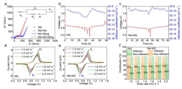
Fig. 4 (a) Nyquist plots and the corresponding fitted curves of NQ and Me-NQ. GITT curves and cation diffusion coefficients of (b) NQ and (c) Me-NQ. CV curves of (d) NQ and (e) Me-NQ cathodes at various scan rates, and (f) the calculated non-diffusion-controlled and diffusion-controlled contributions at various scan rates.
