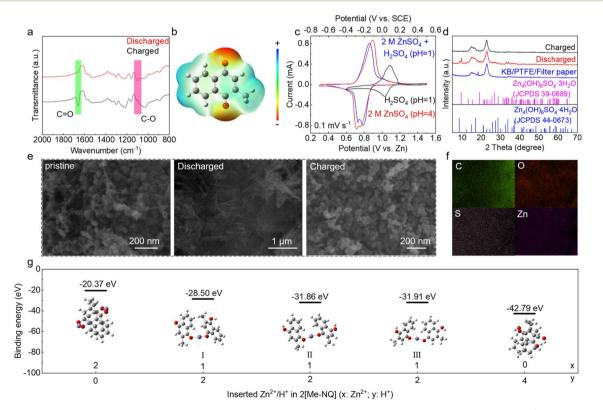
Fig. 5 (a) FT-IR of Me-NQ at different states. (b) ESP map of Me-NQ. (c) CV of Me-NQ in different electrolytes at  $0.1 \,\mathrm{mV} \,\mathrm{s}^{-1}$ . (d) XRD patterns and (e) SEM images of Me-NQ at different states. (f) EDS mappings of the discharged Me-NQ. (g) Binding energies of two Me-NQ molecules with different numbers of  $\mathrm{Zn}^{2+}$  and  $\mathrm{H}^+$ .
