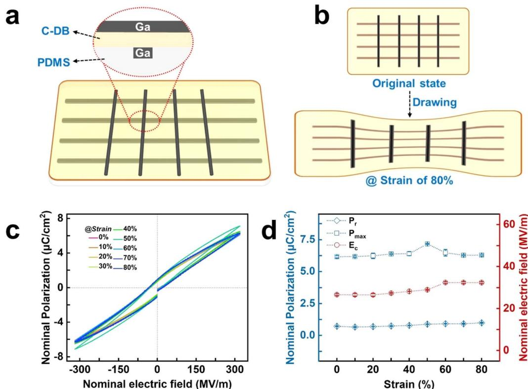
Fig. 5 FE response of elastic RFEs under strains. (a and b) Schematic structure of elastic device (a) in the stretching set-up under 0 and 80% strain (b). (c)  $P$ - $E$  loops at 1 kHz under strain from 0 to 80%. (d)  $P_r$ ,  $P_{\text{max}}$ , and  $E_c$  under different strains.
