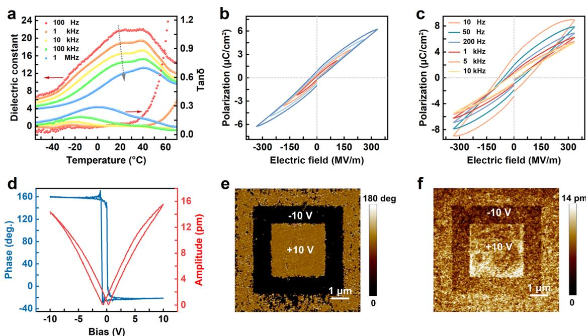
Fig. 4 Ferroelectric properties of crosslinked P(VDF-CTFE-DB) films. (a) Temperature-dependent  $\epsilon$  and dielectric loss of crosslinked P(VDF-TrFE-DB) films at different frequencies. (b and c)  $P$ - $E$  loops of Au/C-P(VDF-CTFE-DB)/Au under different electric fields at 1000 Hz (b) and different frequencies (c). (d) Phase-voltage hysteresis and amplitude-voltage butterfly loop. (e and f) phase (e) and amplitude (f) mapping of PFM.
