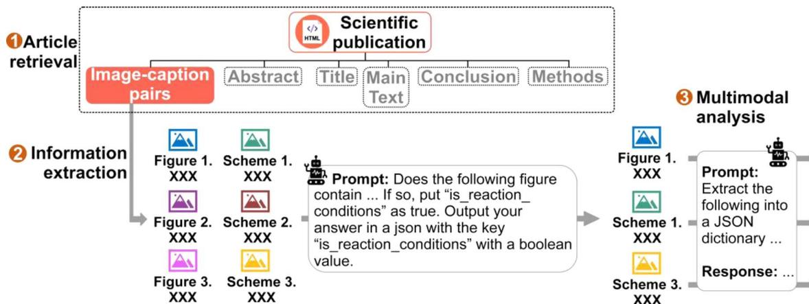
Fig. 6 Schematic illustration of multimodal pipeline for automated reaction mining featuring three sequential steps: article retrieval, information extraction, and multimodal analysis of filtered information.
