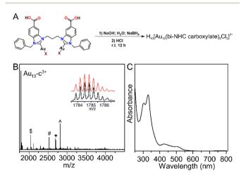
Fig. 1 (A) Preparation of the  $Au_{13}$ -c cluster; (B) FTICR-MS profile of the crude reaction mixture dissolved in DMF. From right to left: (\$)  $H_{12}[Au_{13}$ -c +  $Au(NHC)Cl^{3+}$ , (#)  $H_{8}[Au_{13}(NHC)_4Cl_3Au_1H_5]^{2+}$ , (\*)  $H_{10}[Au_{13}$ -c +  $Cl^{2+}$ , (^)  $H_{10}[Au_{13}$ -c +  $AuCl_2l^{2+}$ . Inset: simulated (red curve) and experimental (black curve) isotope distribution patterns; (C) UV-Vis spectrum recorded of the  $Au_{13}$ -c cluster.
