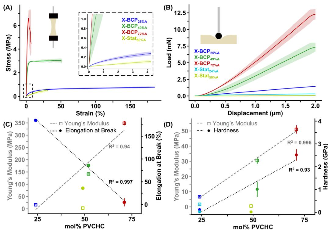
Fig. 5 Mechanical properties of each BCP and Stat<sub>50%A</sub> printed objects. (A) Tensile stress/strain curve from DMA with a zoomed inset ( $n = 3$ ); (B) nanoindentation plot of load vs. displacement ( $n = 3$ ). (C) Tensile properties (Young's modulus and elongation at break) compared to mol% PVCHC. (D) Nanoindentation properties (Young's modulus and hardness) compared to mol% PVCHC.
