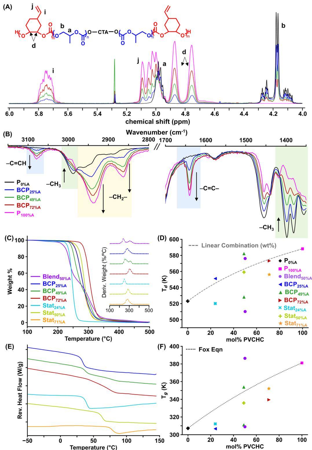
Fig. 2 Chemical and thermal characterization of polymer samples. (A)  $^1\text{H}$  NMR spectroscopy. (B) FTIR spectroscopy. (C) TGA with inset showing the first derivatives; (D)  $T_d$  as a function of mol% PVCHC; (E) MDSC showing the offset normalized reversing heat flow trace; and (F)  $T_g$  as a function of mol% PVCHC.
