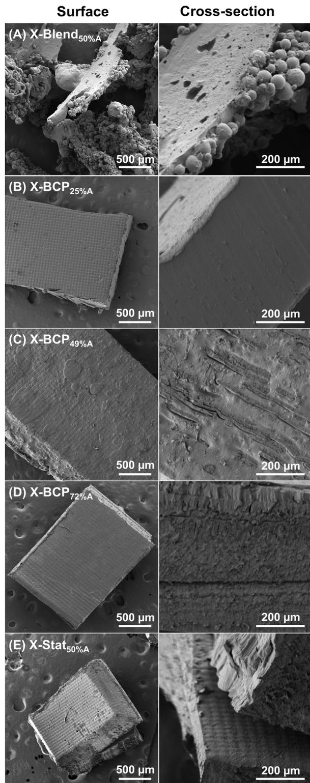
Fig. 4 SEM of surface (left) and cross-section (right) of each printed object after drying: (A) X-Blend<sub>50%A</sub>, (B) X-BCP<sub>25%A</sub>, (C) X-BCP<sub>49%A</sub>, (D) X-BCP<sub>72%A</sub>, and (E) X-Stat<sub>50%A</sub>.
