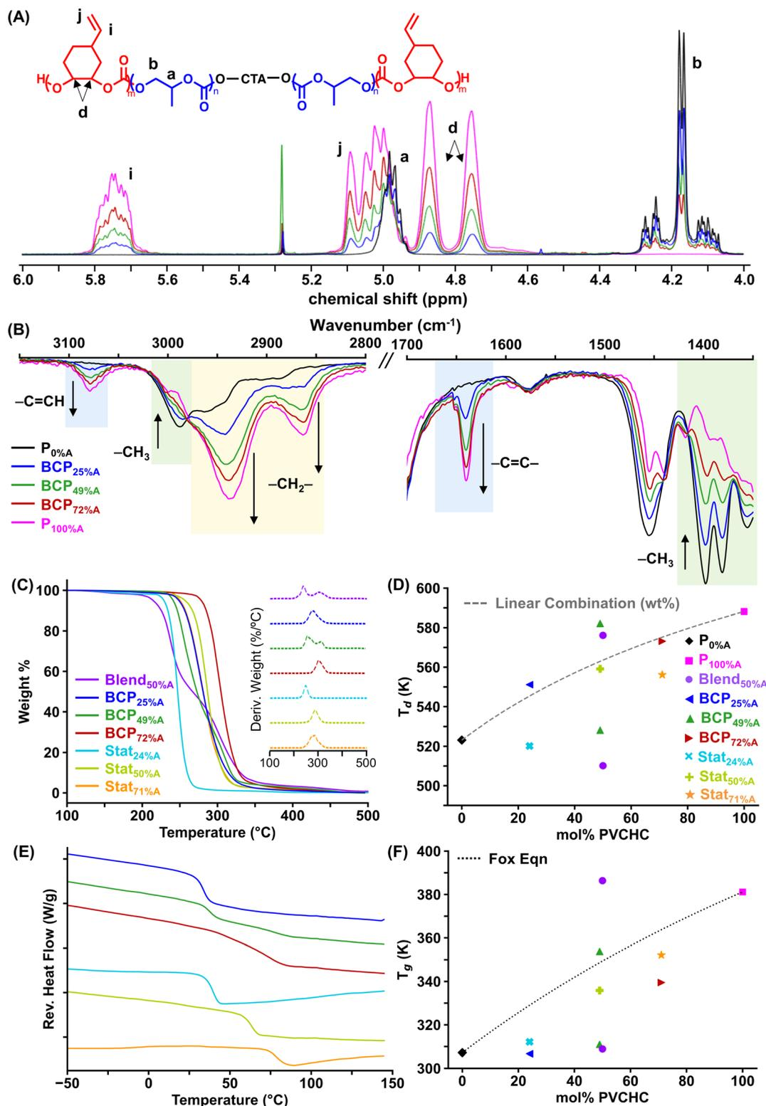
Fig. 2 Chemical and thermal characterization of polymer samples. (A)  $^1\text{H}$  NMR spectroscopy. (B) FTIR spectroscopy. (C) TGA with inset showing the first derivatives; (D)  $T_g$  as a function of mol% PVCHC; (E) MDSC showing the offset normalized reversing heat flow trace; and (F)  $T_g$  as a function of mol% PVCHC.
