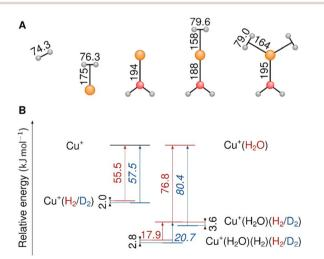
Fig. 3 (A) MP2/def2-TZVPP bond lengths (pm) in  $Cu^+(H_2)$ ,  $Cu^+(H_2O)$  and  $Cu^+(H_2O)(H_2)_{1,2}$  (colours: Cu orange, O red, H grey). (B) MP2/def2-TZVPP dissociation energies (kJ  $mol^{-1}$ ) with anharmonic (VPT2) ZPE correction. The red values (blue values in italic font) represent the dissociation energies of  $H_2$  ( $D_2$ ). Dissociation ZPE differences are highlighted.
