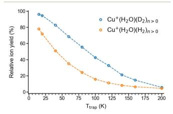
**Fig. 1** Total relative ion yield of  $Cu^+(H_2O)(H_2)_{n>0}$  and  $Cu^+(H_2O)(D_2)_{n>0}$  for ion trap temperatures ranging from 15 K to 200 K, obtained from the TOF mass spectra shown in Fig. S1.† The TOF mass spectra were recorded after storing  $Cu^+(H_2O)$  cations on average 50 ms in a temperature-controlled ion trap filled with roughly 1 mbar of  $H_2$  or  $D_2$ .
