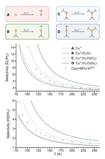
Fig. 5 Predicted selectivities for dihydrogen isotopologue adsorption at  $Cu^+$ ,  $Cu^+(H_2O)$ , and  $Cu^+(H_2O)(H_2)$  as a function of temperature. For the latter, two models are compared (see text). Literature data of Cu(i)-MFU-4l are shown for comparison.<sup>4</sup>
