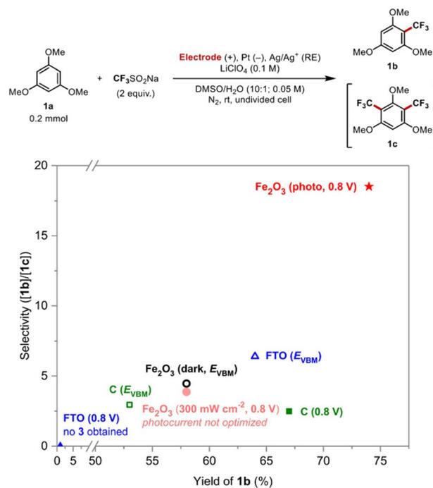
Fig. 7 Reaction yield and selectivity depending on electrode material and applied voltage.  $E_{\text{VBM}}$  corresponds to the valence band edge of hematite, 1.8 V vs. Ag/Ag<sup>+</sup>.
