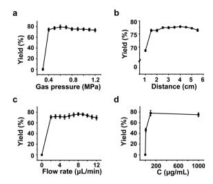
Fig. 2 Effects of microdroplet working conditions on the yields of hydroxylation products of N,N-dimethylaniline (DMA) at m/z 138. (a) Yields as a function of gas pressure. (b) Yields as a function of the distance between the tip of the capillary tube and the MS inlet. (c) Yields as a function of the flow rate of the aqueous DMA solution. (d) Yields as a function of the concentration of the aqueous DMA solution.
