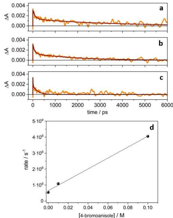
Fig. 4 Normalized temporal evolution of ΔA measured at 1440 nm (orange line) for a degassed solution of 4CzIPN<sup>•-</sup> (a) and in the presence of 0.01 M (b) and 0.1 M (c) 4-bromoanisole. (d) Rate constant of the ΔA decay at 1440 nm as a function of the concentration of 4-bromoanisole.
