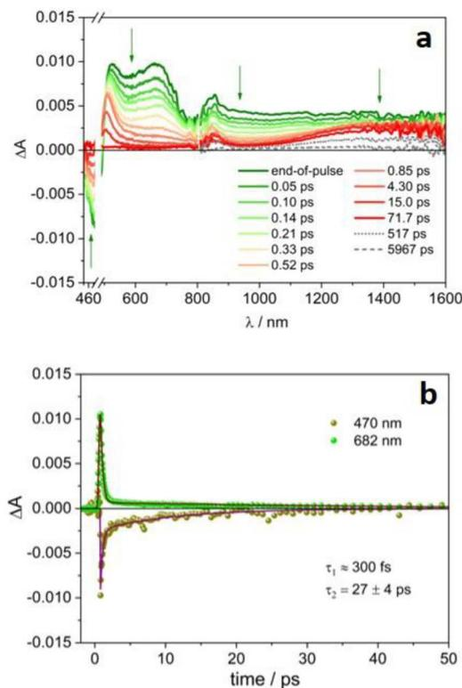
Fig. 3 Transient absorption spectra at different delays of a degassed acetonitrile solution of 4CzIPN<sup>•-</sup> (a) and the corresponding ΔA temporal evolution at significant wavelengths (b). λ<sub>ex</sub> = 480 nm, A<sub>480</sub> = 0.28, 0.2 cm optical path, 8 μJ per pulse.
