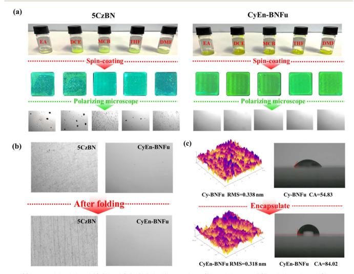
Fig. 3 (a) Images of dissolution of 5CzBN and CyEn-BNFu in different solvents (EA = ethyl acetate, DCE = dichloroethane, MCB = monochlorobenzene, THF = tetrahydrofuran, DMF = N,N-dimethylformamide); spin-coating pictures and corresponding polarized light microscope images. (b) Polarized light microscopy images of 5CzBN and CyEn-BNFu before and after bending. (c) Atomic force microscope (AFM) images and contact angles of Cy-BNFu and CyEn-BNFu.
