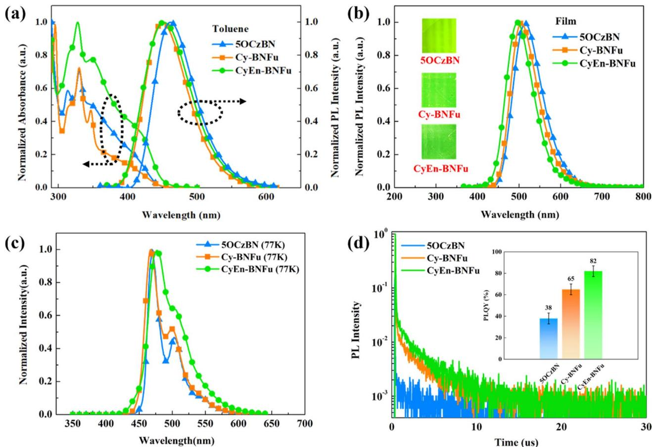
Fig. 2 (a) UV-vis absorption and PL emission of 5OCzBN, Cy-BNFu and CyEn-BNFu in toluene ( $10^{-4}$  M) at room temperature. (b) PL emission of 5OCzBN, Cy-BNFu and CyEn-BNFu in toluene states. (c) Phosphorescence spectra at 77 K of 5OCzBN, Cy-BNFu and CyEn-BNFu in toluene ( $10^{-4}$  M). (d) Transient PL spectra of 5OCzBN, Cy-BNFu and CyEn-BNFu in the pure films (the inset shows the PLQY of 5OCzBN, Cy-BNFu and CyEn-BNFu in pure films).
