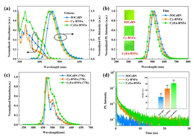
Fig. 2 (a) UV-vis absorption and PL emission of 5OCzBN, Cy-BNFu and CyEn-BNFu in toluene ( $10^{-4}$  M) at room temperature. (b) PL emission of 5OCzBN, Cy-BNFu and CyEn-BNFu in toluene states. (c) Phosphorescence spectra at 77 K of 5OCzBN, Cy-BNFu and CyEn-BNFu in toluene ( $10^{-4}$  M). (d) Transient PL spectra of 5CzBN, Cy-BNFu and CyEn-BNFu in the pure films (the inset shows the PLQY of 5OCzBN, Cy-BNFu and CyEn-BNFu in pure films).
