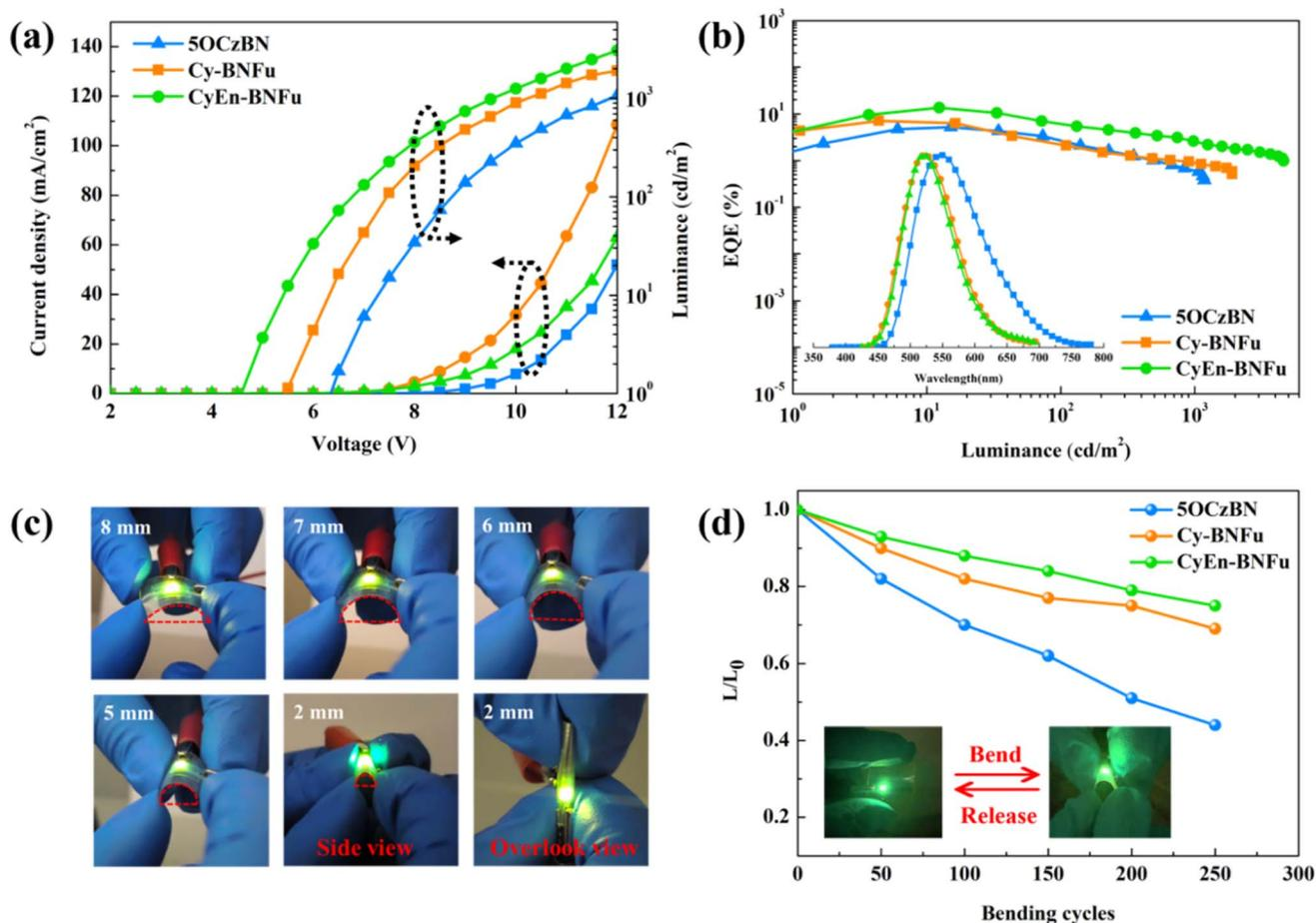
Fig. 5 (a) Current density–voltage–luminance ( $J$ – $V$ – $L$ ) curves of 5OCzBN, Cy-BNFu and CyEn-BNFu OLEDs. (b) External quantum efficiency (EQE) versus luminance. Inset: The photo of the EL spectra. (c) Emission images of the PET-based OLED captured at high luminance (>3000 cd m<sup>-2</sup>) under random deformation and with decreasing bending radii from 8 to 2 mm at 7 V. (d) Luminance of the flexible OLEDs as a function of the bending radius after 250 bending cycles.
