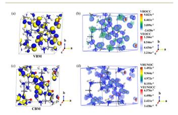
Fig. 6 The electron distribution profiles of  $N_2H_4Zn(HC_3N_3O_3)$ : the (a) VBM and (c) CBM. SHG weight factor analysis of the  $d_{11}$  component of the  $N_2H_4Zn(HC_3N_3O_3)$  crystal (b) and (d).
