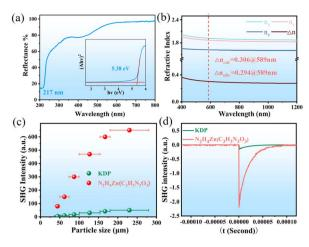
Fig. 2 Optical properties of N<sub>2</sub>H<sub>4</sub>Zn(HC<sub>3</sub>N<sub>3</sub>O<sub>3</sub>): (a) UV-vis diffuse reflectance spectrum; inset: the experimental band gap calculated with the Kubelka-Munk functional. (b) The calculated refractive indices. (c) Particle-size-dependent SHG intensity under 1064 nm laser irradiation (d) Oscilloscope traces of the SHG signals for polycrystalline samples with a particle size range of 180-280 μm.
