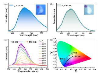
Fig. 4 The phosphorescence spectra of  $N_2H_4Zn(HC_3N_3O_3)$ . The emission spectra at (a) 310 nm; (b) 365 nm. (c) The emission spectrum from 290 to 410 nm. (d) CIE color chromaticity under excitation from 310 to 365 nm
