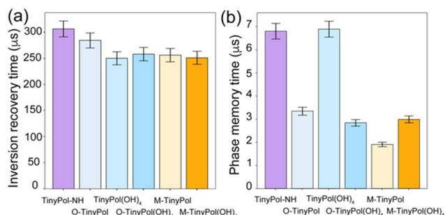
Fig. 2 (a) Electron inversion recovery time ( $T_{ir}$ ) and (b) electron phase memory time ( $T_m$ ), for the six radicals investigated here. The electron relaxation parameters were measured at W band at 105 K using 100  $\mu$ M solutions in  $d_8$ -glycerol/D<sub>2</sub>O/H<sub>2</sub>O 60/30/10 (v/v/v).
