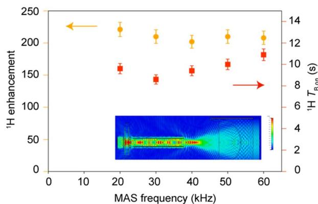
Fig. 6 Enhancement factors and polarization build-up times of 10 mM M-TinyPol(OH)<sub>4</sub> in a bulk solution of  $d_8$ -glycerol/ $D_2O$ / $H_2O$  60/30/10 (v/v/v), as a function of MAS frequency. Enhancements values were measured at 18.8 T from proton NMR spectra, in a 0.7 mm zirconia rotor at a sample temperature of  $110 \pm 5$  K. The inset shows the microwave distribution within the rotor predicted by finite-element simulations.
