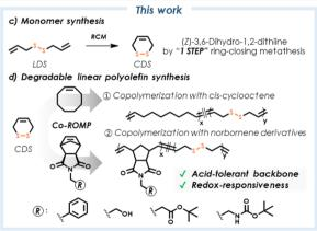
Fig. 1 Synthesis of disulfide-containing polyolefins by ROMP: (a) prior multistep synthesis of the 8-membered disulfide-containing cyclic olefin, (*Z*)-3,4,7,8-tetrahydro-1,2-dithiocine and (b) its copolymerization with cyclic olefins; (c) ring-closing metathesis (RCM) of LDS affords (*Z*)-3,6-dihydro-1,2-dithiine (CDS); (d) CDS copolymerization with *cis*-cyclooctene or norbornene derivatives gives entry into disulfide-containing polyolefins by ROMP.
