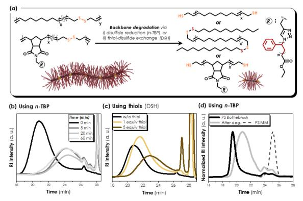
Fig. 6 (a) P-20-k and PS BP-10 degradation by (i) reduction of disulfide or (ii) thiol-disulfide exchange; SEC curves eluting with THF of (b) P-20-k reduction of disulfide with n-TBP, (c) P-20-k thiol-disulfide exchange with 1-dodecanethiol, and (d) PS BP degradation by n-TBP as a reducing agent before and after disulfide reduction.
