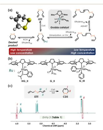
Fig. 2 (a) Metathesis CDS–LDS equilibria; (b) chemical structures of the ruthenium benzylidene catalysts employed in this work; (c) <sup>1</sup>H NMR spectra of LDS and CDS (from Entry 3 in Table 1).
