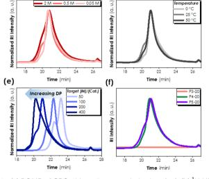
Fig. 5 (a) ROMP of CDS with norbornene derivatives 1-4; (b)  $^1H$  NMR spectrum of P1-20 from Entry 2 in Table 3; SEC curves with variation of (c) total monomer concentration at [1]: [CDS] = 4:1 with [monomer]/[initiator] ratio at 200; (d) temperature; (e) [monomer]/[initiator] at 2 M monomer and [1]: [CDS] = 4:1; and (f) ROMP copolymerization of CDS with norbornene derivatives with containing pendent, hydroxy, t-butyl ester, and t-boc amine groups.
