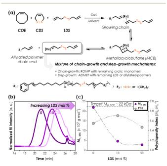
Fig. 4 (a) Copolymerization of COE/CDS/LDS mixture; (b) SEC (eluting with THF) curves resulting from polymerizations with 0, 10, or 20 mol% LDS; (c) Plot of  $M_{\rm n, SEC}$  and PDI vs. LDS mol%.
