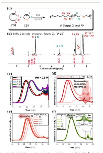
Fig. 3 (a) ROMP copolymerization of COE and CDS; (b)  $^1$ H NMR spectrum of P-20 from Entry 2 in Table 2; SEC curves eluting with THF with various (c) CDS mol% while fixing [monomer]/[initiator] ratio at 200, (d) total monomer concentration at [COE]: [CDS] = 4:1 with [monomer]/[initiator] ratio at 200, (e) [monomer]/[initiator] at [monomer] = 2 M and [COE]: [CDS] = 4:1, and (f) impact of reaction time following introduction of G\_III.
