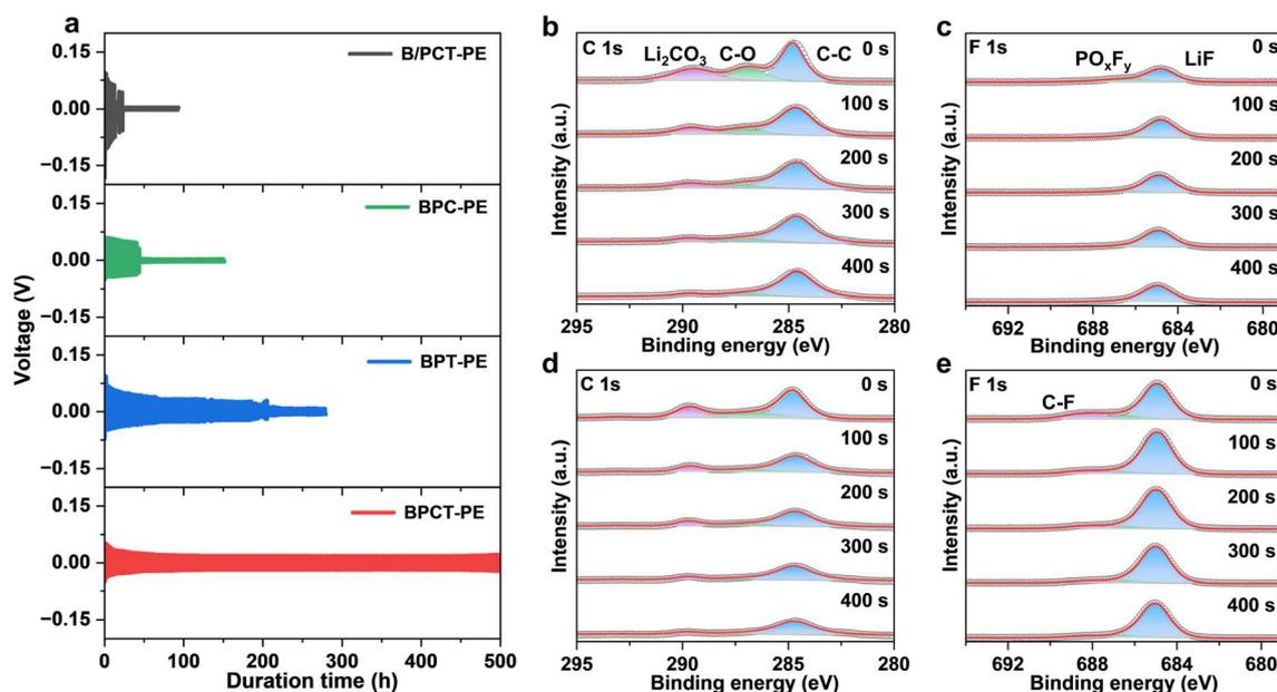
Fig. 4 (a) Voltage profiles of Li/Li symmetric cells with BPCT-PE and control samples, including B/PCT-PE, BPC-PE and BPT-PE at  $0.5 \text{ mA cm}^{-2}$  and  $0.5 \text{ mA h cm}^{-2}$ . (b–e) The high-resolution C 1s and F 1s spectra obtained from XPS depth measurement of the SEI formed in (b and c) BPC-PE and (d and e) BPCT-PE at  $0.1 \text{ mA cm}^{-2}$  and  $0.1 \text{ mA h cm}^{-2}$  after 100 cycles.
